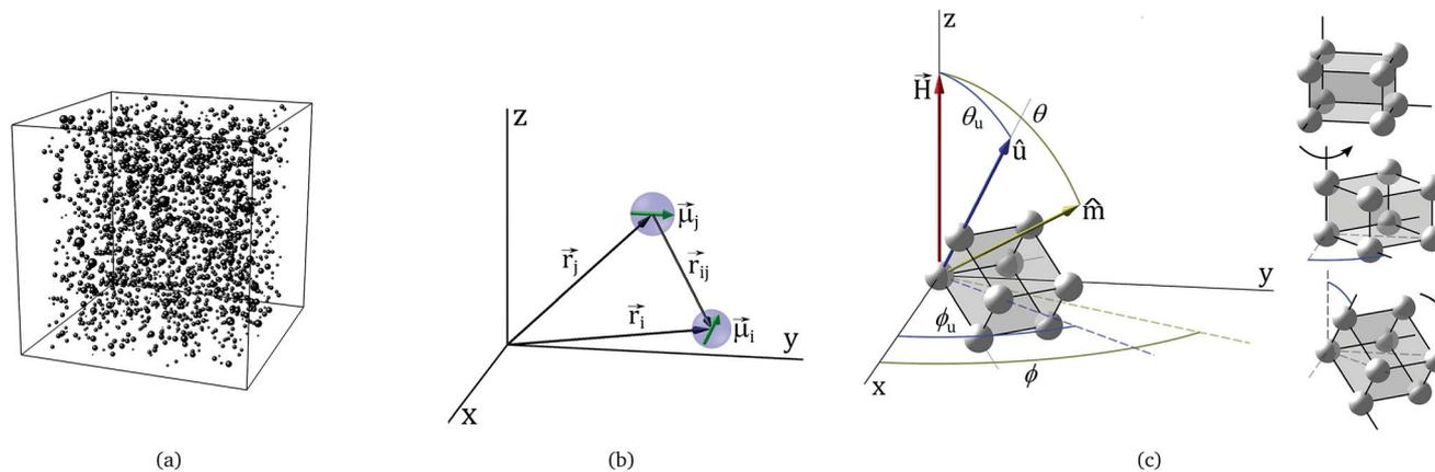
Fig. 1 Coordinate system adopted. In (a), we depict a box simulation containing 2000 particles, with  $c = 10^{-2}$ , and in (b), we present the quantities of interest for the dipolar field calculations. In (c), we illustrate the process of coordinate rotations used to transform the cosine directions of the anisotropic energy to the box simulation coordinate system.
