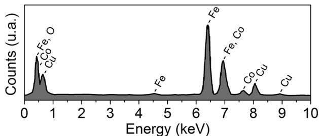
Fig. 3 The EDS spectrum of the CoFe<sub>2</sub>O<sub>4</sub> nanopowder.
