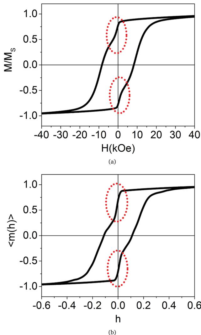
Fig. 10 (a) Experimental results for the isothermal magnetic hysteresis of  $\text{CoFe}_2\text{O}_4$  ( $T = 5$  K) and (b) the theoretical results. The red dots represent the region of curves in which the magnetization abruptly changes.
