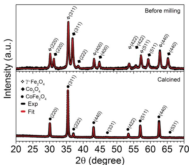
Fig. 2 The XRD patterns, including the Rietveld refinement (red solid line) of the precursor powders before milling and the  $\text{CoFe}_2\text{O}_4$  sample indexed with the  $(hkl)$  reflections of the spinel structure.
