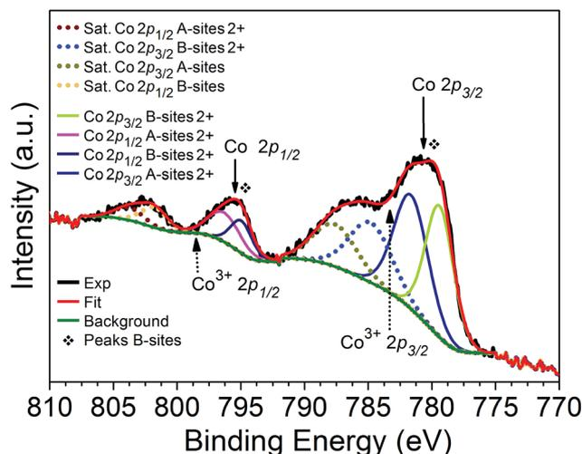
Fig. 8 XPS high resolution spectra of Co 2p of the  $\text{CoFe}_2\text{O}_4$  nanopowder. Dashed arrows indicate the expected values<sup>29</sup> of the binding energies of the  $\text{Co}^{3+}$  species in octahedral (783.3 eV) and tetrahedral sites (798.5 eV). Dashed lines correspond to shake-up satellite peaks.
