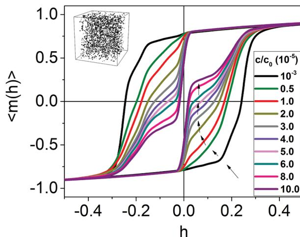
Fig. 9 Reduced magnetic hysteresis curves for different values of  $c/c_0$ , with  $N = 2000$  and  $\sigma = 0.3$ . The black arrows indicate the formation of "jumps" in the reduced hysteresis as  $c/c_0$  increases.
