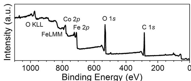
Fig. 6 XPS survey spectrum of the  $\text{CoFe}_2\text{O}_4$  nanopowder.
