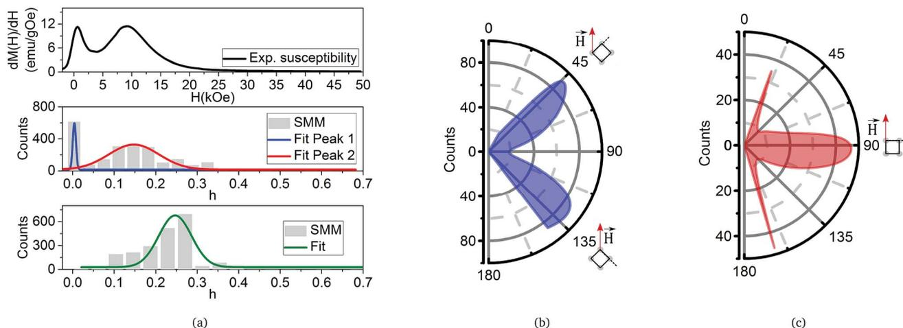
**Fig. 11** In (a) (top), we show the experimental isothermal susceptibility  $\frac{dM(H)}{dH}$ , (middle) the SMM histogram for the simulation with  $c/c_0 = 3.5 \times 10^{-5}$  showing the two-peak fits of the histogram, and (bottom) the SMM histogram for a very diluted sample with  $c/c_0 = 10^{-8}$  (very weak dipolar interactions) showing only one peak. In (b), we show a polar distribution of SMMs around peak 1 and (c) the polar distribution of SMMs around peak 2.
