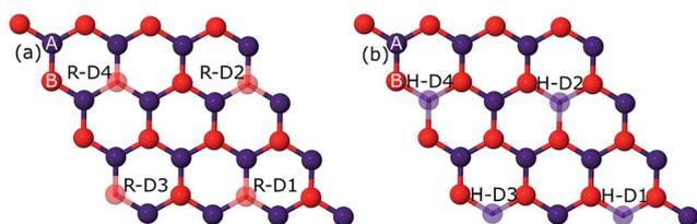
Fig. 1 The red hollow spheres, denoted by RD1–RD4, corresponding to rectangular doping are presented in (a). The hexagonal configuration is shown by the blue hollow spheres (HD1–HD4) pictured in (b). A and B indicate the sublattice sites A and B.
