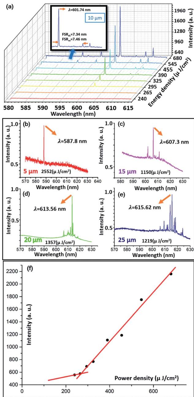
Fig. 3 (a) Lasing spectra of the microsphere with a diameter of 10  $\mu\text{m}$  under different pumping energies (waterfall) (insets: detailed information for the spectrum under the pump of 545  $\mu\text{J cm}^{-2}$  energy density). (b–e) Lasing spectra from microspheres with diameters of 5  $\mu\text{m}$ , 15  $\mu\text{m}$ , 20  $\mu\text{m}$ , 25  $\mu\text{m}$  under the appropriate energy density respectively. (f) The lasing threshold characteristic in (a).
