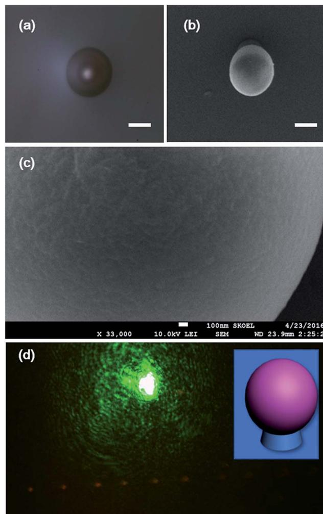
Fig. 2 (a) Top-view optical microscopic images of 10  $\mu\text{m}$  microsphere laser, scale bar: 10  $\mu\text{m}$ . (b, c) SEM image of 10  $\mu\text{m}$  microsphere laser, scale bar: (b) 1  $\mu\text{m}$ ; (c) 100 nm. (d) Microspheres measured from CCD, green light: 532 nm pump, (insert: microsphere designed).
