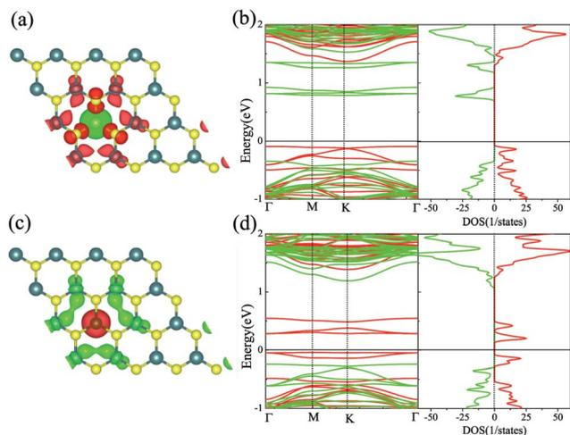
Fig. 1 The structure and SCD of the single Cr (a) and Fe (c) doped monolayer MoS<sub>2</sub>. The isosurface of the SCD is 0.005 e Å<sup>-3</sup>. (b) and (d) are the band structures and DOS for Cr–MoS<sub>2</sub> and Fe–MoS<sub>2</sub>, respectively.
