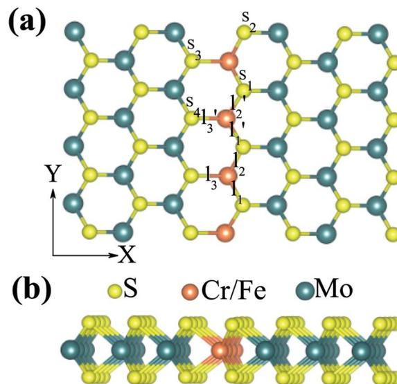
Fig. 2 (a) Top and (b) side view of the δ-type doped monolayer MoS<sub>2</sub>.
