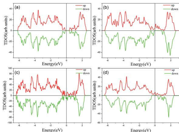
**Fig. 3** The total density of states (TDOS) of Cr and Fe  $\delta$ -type doping in monolayer MoS<sub>2</sub>. The results of FeFe-chain-MoS<sub>2</sub>, CrCr-chain-MoS<sub>2</sub>, FeFeCrCr-chain-MoS<sub>2</sub>, and FeCrFeCr-chain-MoS<sub>2</sub> are shown in (a), (b), (c), and (d), respectively. The Fermi level is set to zero.
