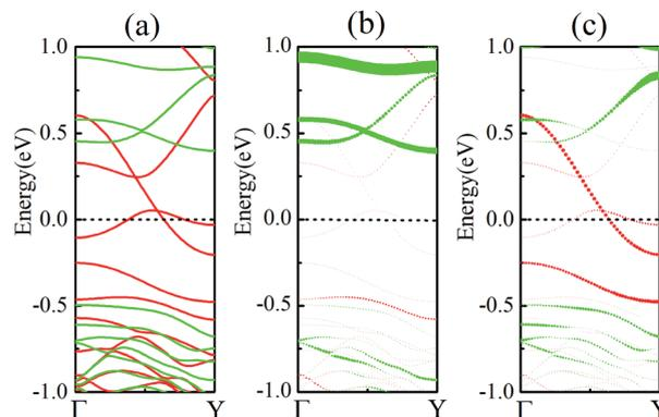
**Fig. 5** (a) Band structures of FeCrFeCr-chain-MoS<sub>2</sub>, with the red and green lines representing the majority and minority spin channels, respectively. The projector of the bands of Cr and Fe are described in (b) and (c), respectively. The Fermi level is set to zero.
