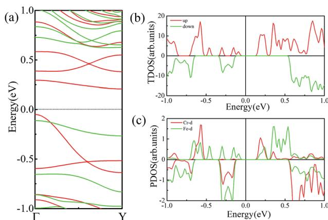
Fig. 8 (a) Band structures of FeCrFeCr-chain-MoS<sub>2</sub> under 12% compression strain. The Fermi level is set to zero. The TDOS and PDOS of Cr and Fe d orbitals are shown in (b) and (c), respectively.
