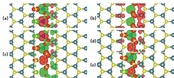
**Fig. 4** The spin charge density (SCD) of CrCr-chain-MoS<sub>2</sub> (a), FeFe-chain-MoS<sub>2</sub> (b), FeFeCrCr-chain-MoS<sub>2</sub> (c), and FeCrFeCr-chain-MoS<sub>2</sub> (d). (e) is the SCD of FeCrFeCr-chain-MoS<sub>2</sub> under 12% compressed strain. The isosurface of the SCD is 0.005 e  $\text{\AA}^{-3}$ . The red and blue isosurfaces denote the majority and minority spin channels, respectively.
