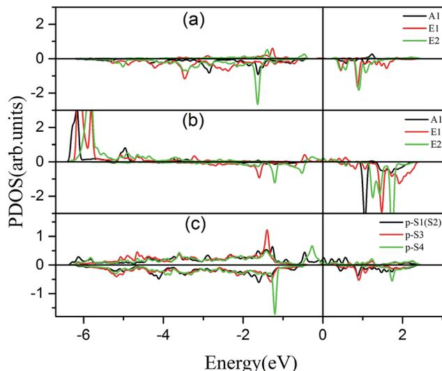
Fig. 6 Partial density of states (PDOS) of the d orbital of Cr (a) and Fe (b). (c) is the PDOS of the p orbitals of S<sub>1(2)</sub>, S<sub>3</sub>, and S<sub>4</sub>. The positive and negative values denote the majority and minority channels, respectively. The Fermi level is set to zero.
