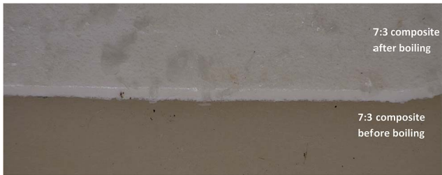
Fig. 5 Low resolution microscopy image (24× magnification) showing significant fragmentation of 7 : 3 composite following treatment in boiling water.
