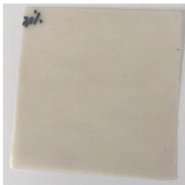
Fig. 3 Representative 7 : 3 m-HDPE : TPS composite.
