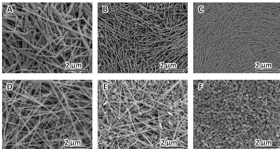
Fig. 4 FE-SEM images of AgNWs synthesized at different [PVP] to [AgNO<sub>3</sub>] molar ratio: (A) 2 : 1, (B) 4 : 1, (C) 6 : 1, (D) 8 : 1, (E) 10 : 1, and (F) 12 : 1.
