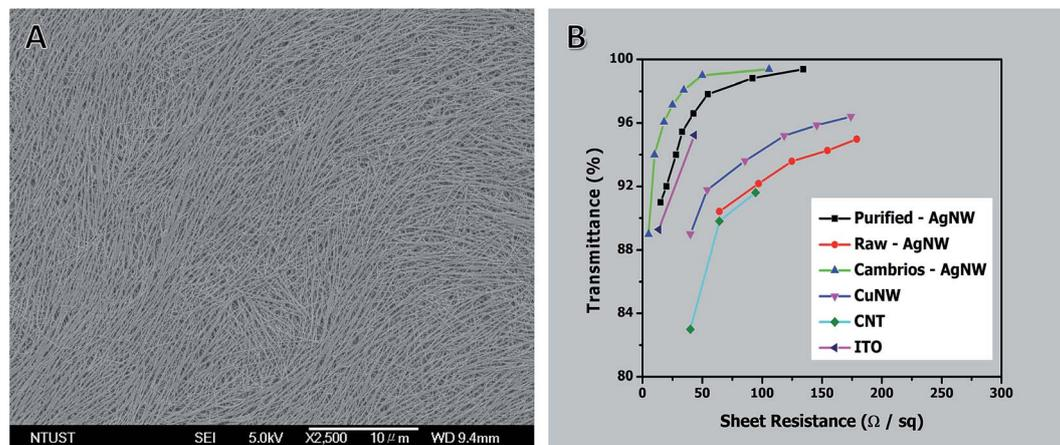
Fig. 8 (A) Typical FE-SEM image of AgNW film. (B) A plot of specular transmittance ( $\lambda = 550$  nm) versus sheet resistance for AgNW films before and after purification. Each data point is the average of five measurements. The performances of AgNWs,<sup>42</sup> CuNWs,<sup>94</sup> CNT,<sup>95</sup> and ITO are shown for comparison.
