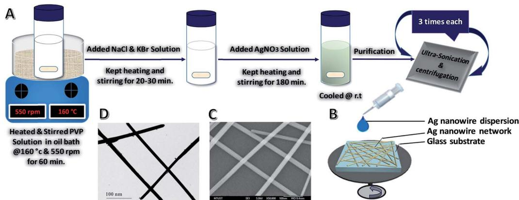
**Fig. 1** (A) Schematic diagram of synthesis and purification of AgNWs with polyol process at 160 °C for 3 h. (B) Schematic diagram of spin-coated AgNW network on a glass substrate. (C) FE-SEM image of the spin-coated AgNW network on the glass substrate. (D) TEM image of the spin-coated AgNW network on a lacey carbon-coated copper grid.
