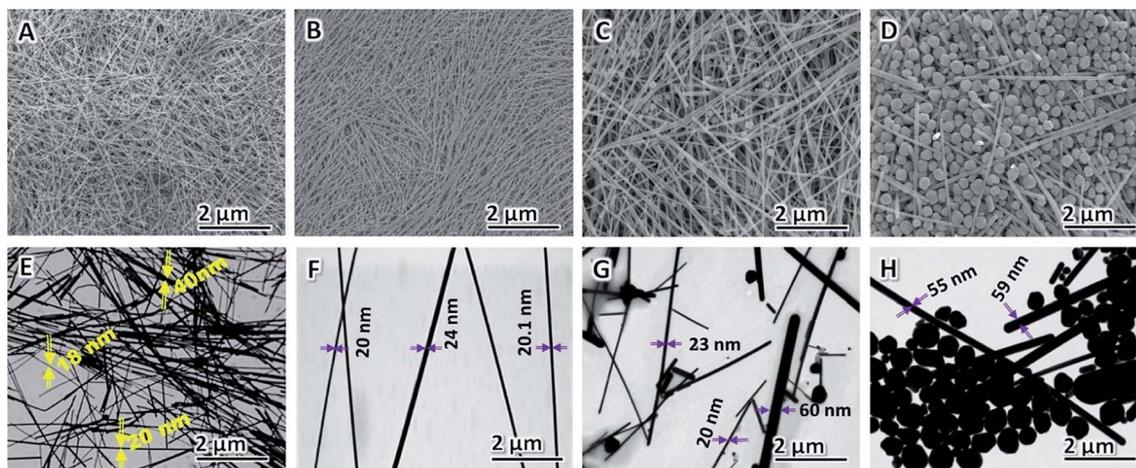
Fig. 3 FE-SEM (A–D) and TEM (E–H) images of purified products obtained from different concentrations of AgNO<sub>3</sub>: (A and E) 20.6, (B and F) 30.5, (C and G) 60.4 and (D and H) 90.3 mM respectively, while the other all parameters were kept constant.
