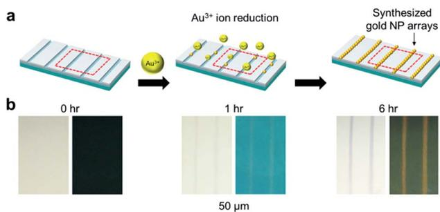
Fig. 2 *In situ* synthesis of gold NPs along the cracked lines on the PDMS substrate. (a) A schematic illustration of the synthesis of gold NPs by crack templated reduction lithography (CTRL). (b) The transmittance (left) and reflection (right) optical images of the perpendicular crack lines at the same region during the 6 h reduction reaction.
