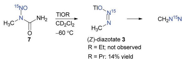
Scheme 2 Synthesis of diazotate 3 and subsequent decomposition to CH 2 N 15 N.
