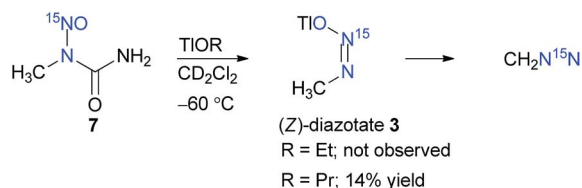
Scheme 2 Synthesis of diazotate 3 and subsequent decomposition to CH 2 N 15 N.
