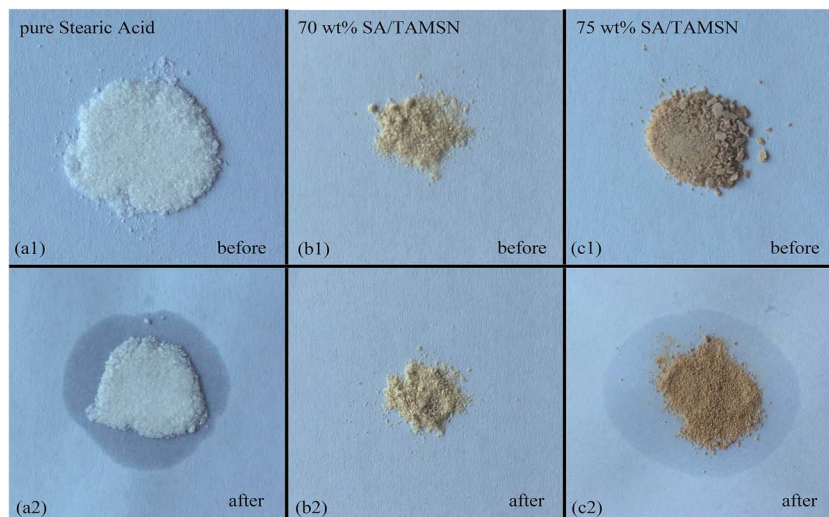
Fig. 7 Leakage test photographs of stearic acid, 70 wt% SA/TAMSN and 75 wt% SA/TAMSN.
