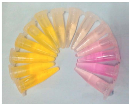
Fig. 2 Color changes of sensor 1 in ethanol–water (1 : 10, v/v) measured as a function of pH.
