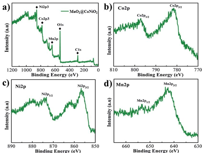
Fig. 4 XPS spectrum of  $\text{MnO}_2@CoNiO_2$  on Ni-foam; (a) survey spectrum, high-resolution spectra for (b) Co 2p, (c) Ni 2p, and (d) Mn 2p.
