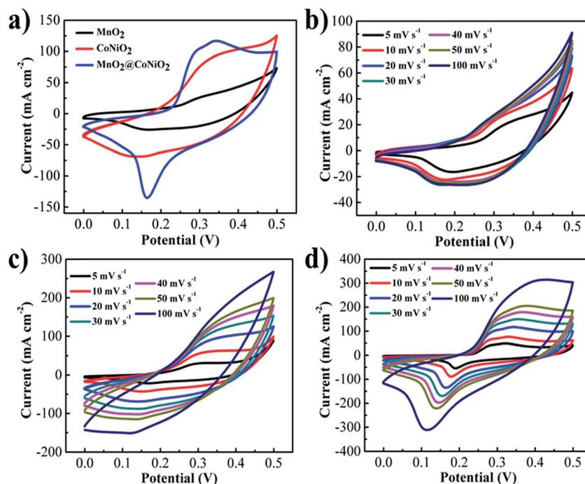
Fig. 6 (a) A comparison CV curves of the  $\text{MnO}_2$ ,  $\text{CoNiO}_2$  and  $\text{MnO}_2@\text{CoNiO}_2$  electrodes at the scan rate of  $20 \text{ mV s}^{-1}$ . CV curves of the (b)  $\text{MnO}_2$ , (c)  $\text{CoNiO}_2$  and (d)  $\text{MnO}_2@\text{CoNiO}_2$  electrodes at different scan rates ( $5\text{--}100 \text{ mV s}^{-1}$ ) in  $3 \text{ M KOH}$  solution.
