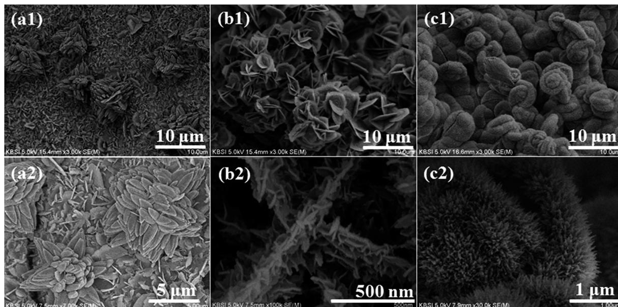
Fig. 1 (a1, b1 and c1) high magnification and (a2, b2 and c2) low magnification typical FE-SEM images of the (a1 and a2)  $\text{MnO}_2$ , (b1 and b2)  $\text{CoNiO}_2$  and (c1 and c2)  $\text{MnO}_2@CoNiO_2$  electrodes.
