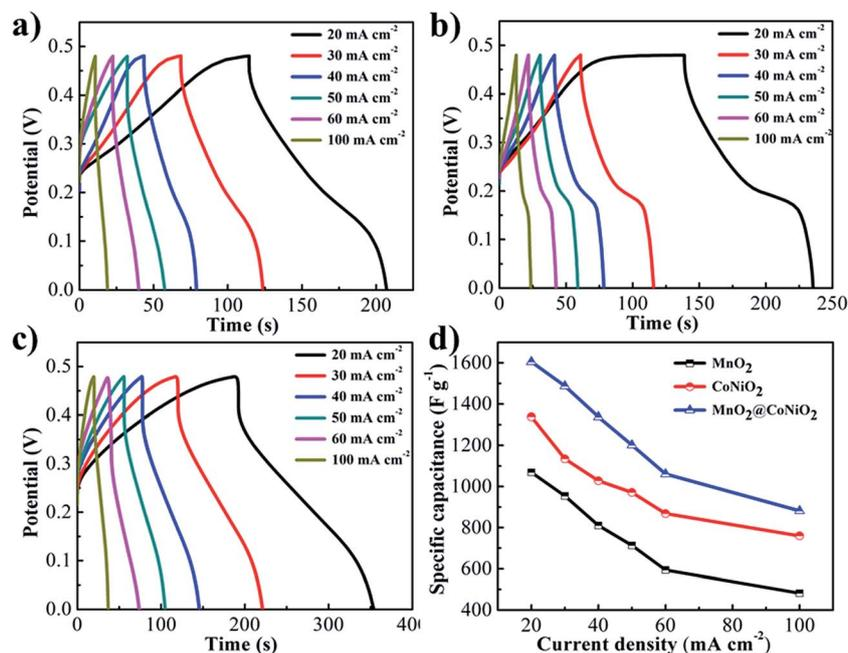
Fig. 7 Charge and discharge curves of the (a)  $\text{MnO}_2$ , (b)  $\text{CoNiO}_2$  and (c)  $\text{MnO}_2@\text{CoNiO}_2$  electrodes at different current densities ( $20\text{--}100 \text{ mA cm}^{-2}$ ) in  $3 \text{ M KOH}$  solution; (d) the measured specific capacitance as a function of current density.
