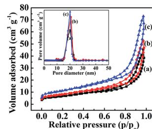
Fig. 5 The Brunauer-Emmett-Teller (BET) surface area measured from nitrogen adsorption-desorption isotherms and the insets show the corresponding pore-size distribution of the (a)  $MnO_2$ , (b)  $CoNiO_2$  and (c)  $\text{MnO}_2@CoNiO_2$  on Ni-foam substrate.
