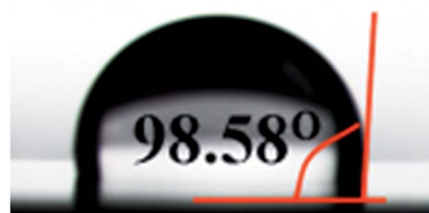
Fig. 6 Contact angle of water on a PD 1 film.
