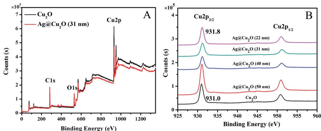
Fig. 4 XPS spectra. (A) Survey spectra of Cu<sub>2</sub>O nanospheres and Ag@Cu<sub>2</sub>O (31 nm). (B) Cu2p peak regions of Cu<sub>2</sub>O nanospheres and Ag@Cu<sub>2</sub>O core-shell NPs samples with various Cu<sub>2</sub>O shell thickness.
