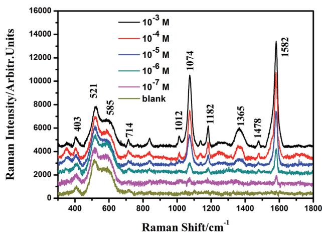
Fig. 7 Concentration-dependent ( $10^{-3}$ ,  $10^{-4}$ ,  $10^{-5}$ ,  $10^{-6}$ ,  $10^{-7}$  M, and blank sample) SERS spectra of 4-MBA adsorbed on the Ag@Cu<sub>2</sub>O core-shell NPs samples with the Cu<sub>2</sub>O shell thickness of 31 nm.
