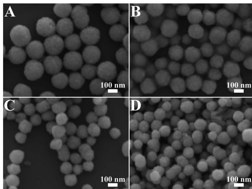
Fig. 2 SEM images of the  $\text{Ag}@\text{Cu}_2\text{O}$  core-shell NPs samples with varying  $\text{Cu}_2\text{O}$  shell thickness. (A)  $\text{Ag}@\text{Cu}_2\text{O}$  (50 nm), (B)  $\text{Ag}@\text{Cu}_2\text{O}$  (40 nm), (C)  $\text{Ag}@\text{Cu}_2\text{O}$  (31 nm), and (D)  $\text{Ag}@\text{Cu}_2\text{O}$  (22 nm).
