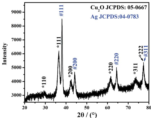
Fig. 3 XRD pattern of the Ag@Cu<sub>2</sub>O (31 nm) NPs sample.
