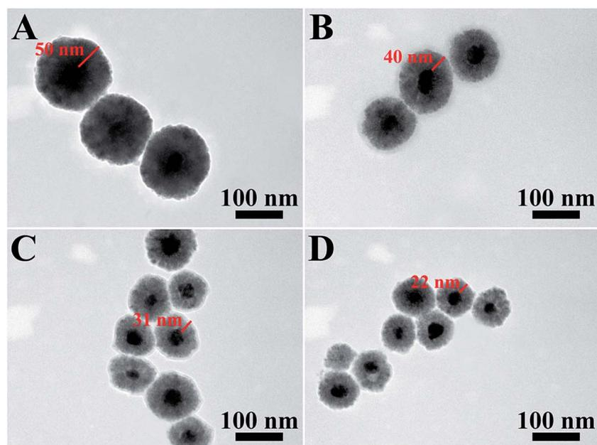
Fig. 1 TEM images of the  $\text{Ag}@\text{Cu}_2\text{O}$  core-shell NPs samples with different  $\text{Cu}_2\text{O}$  shell thickness. (A)  $\text{Ag}@\text{Cu}_2\text{O}$  (50 nm), (B)  $\text{Ag}@\text{Cu}_2\text{O}$  (40 nm), (C)  $\text{Ag}@\text{Cu}_2\text{O}$  (31 nm), and (D)  $\text{Ag}@\text{Cu}_2\text{O}$  (22 nm).
