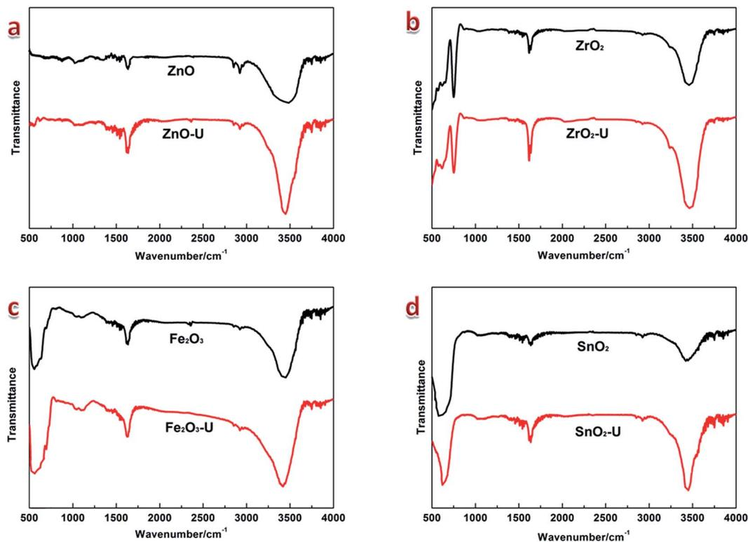
Fig. 3 FTIR spectra of ZnO, ZrO<sub>2</sub>, Fe<sub>2</sub>O<sub>3</sub>, SnO<sub>2</sub> NCs and the corresponding ultrasonic-treated products.
