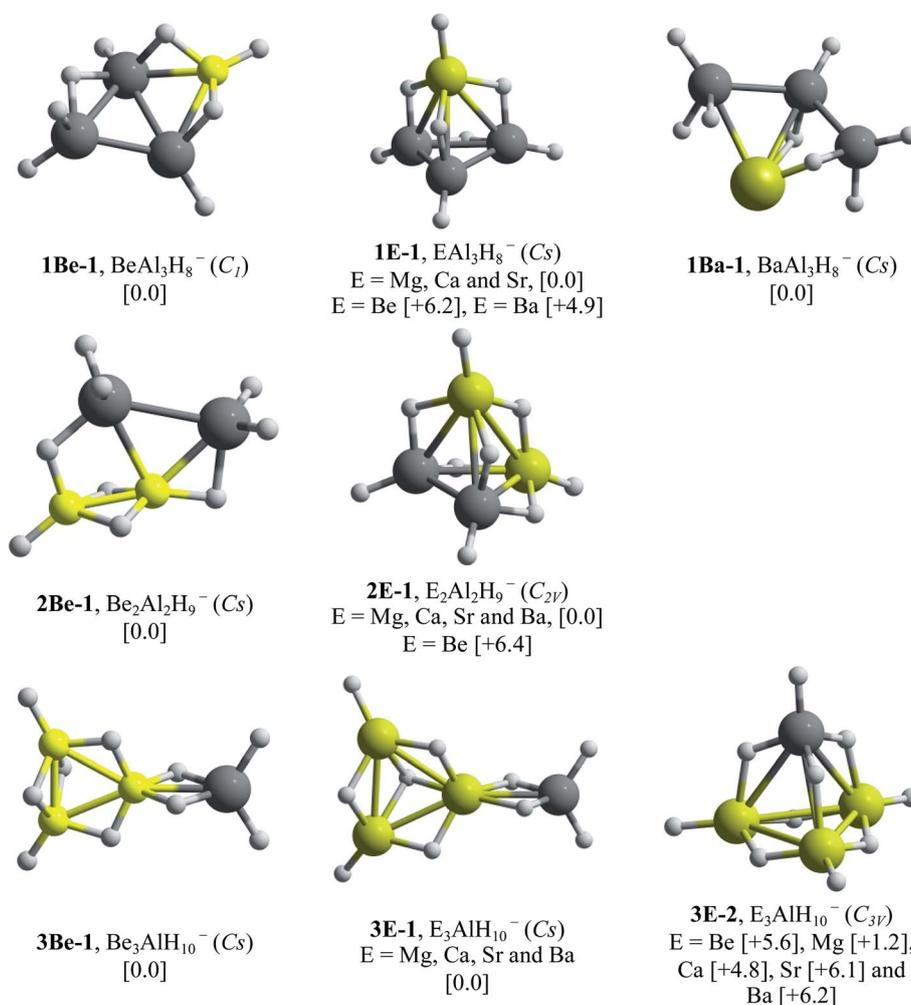
Fig. 2 Lowest energy structures for  $E_n\text{Al}_{4-n}\text{H}_{7+n}^-$  ( $E = \text{Be, Mg, Ca, Sr}$  and  $\text{Ba}$ ) with  $n = 1-3$ . The values in square brackets correspond to relative energies in  $\text{kcal mol}^{-1}$ , among clusters with same composition, obtained at the CCSD(T)/def2-TZVP//PBE0/def2-TZVP level of theory. In all cases, the systems in multiplicity singlet were more stable than the triplet.
