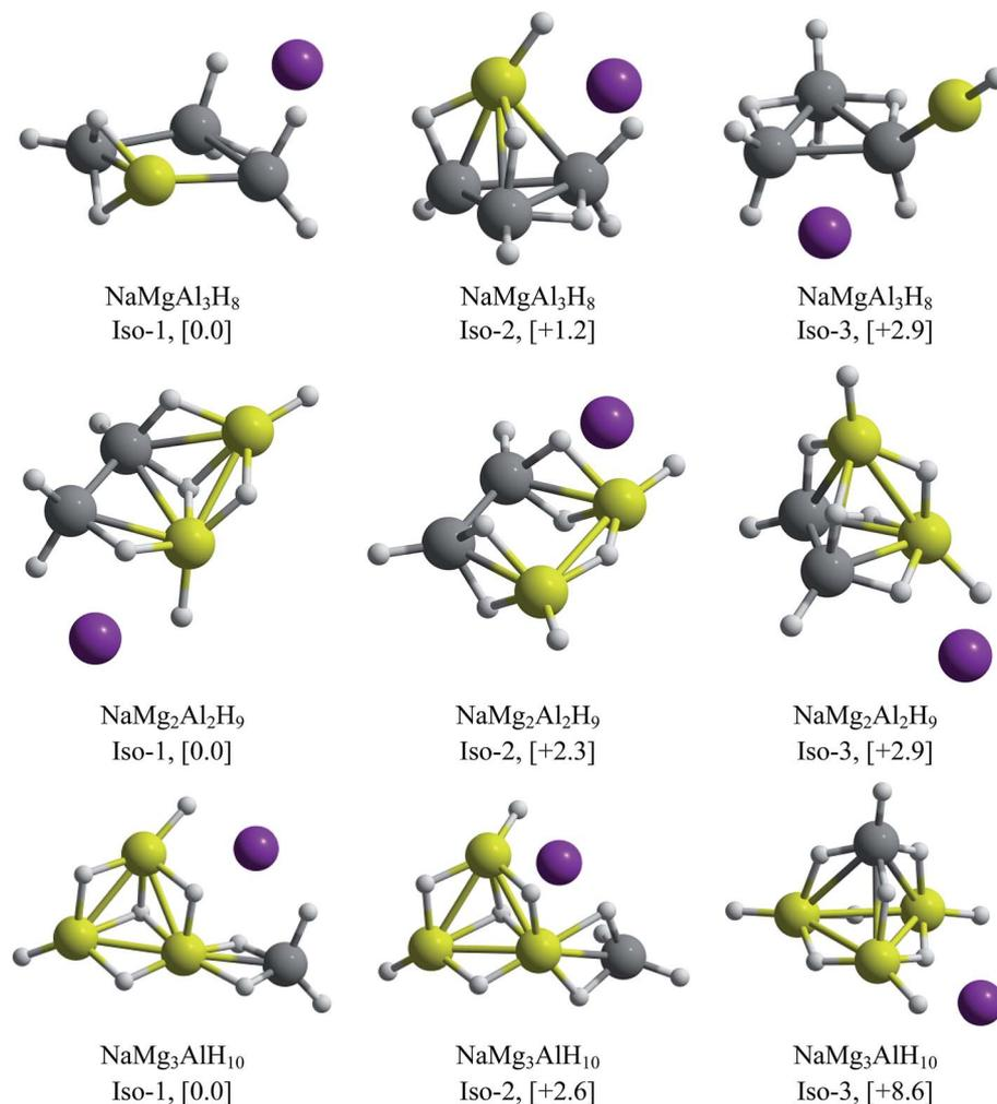
Fig. 8 Lowest energy isomers for NaMgAl<sub>3</sub>H<sub>8</sub>, NaMg<sub>2</sub>Al<sub>2</sub>H<sub>9</sub> and NaMg<sub>3</sub>AlH<sub>10</sub>. The relative energies, in kcal mol<sup>-1</sup> (within squared brackets), were calculated at CCSD(T)/def2-TZVP//PBE0/def2-TZVP level of theory.
