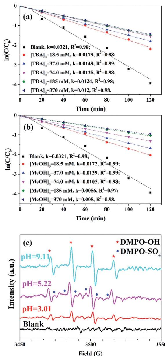
Fig. 7 Pseudo-first-order kinetic curves for AO7 removal by MSDBC/PS system with different scavengers: (a) TBA and (b) MeOH. Reaction conditions: MSDBC dosage = 1.0 g L<sup>-1</sup>, [PS]<sub>0</sub> = 1.85 mM, [AO7]<sub>0</sub> = 0.06 mM and [pH]<sub>0</sub> = 5.22. (c) EPR spectra of MSDBC/PS system under three different pH values (★ represents OH<sup>•</sup> adducts and ● represents SO<sub>4</sub><sup>•-</sup> adducts).
