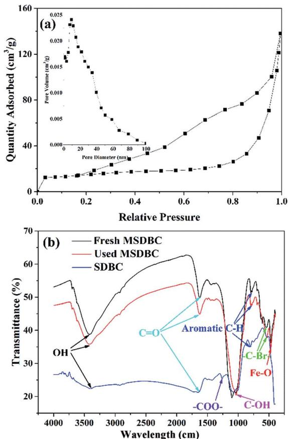
Fig. 3 (a) Nitrogen adsorption–desorption isotherm of MSDBC, insert figure: the corresponding BJH adsorption pore size distribution curve and (b) FTIR spectra of fresh and used MSDBC and SDBC.
