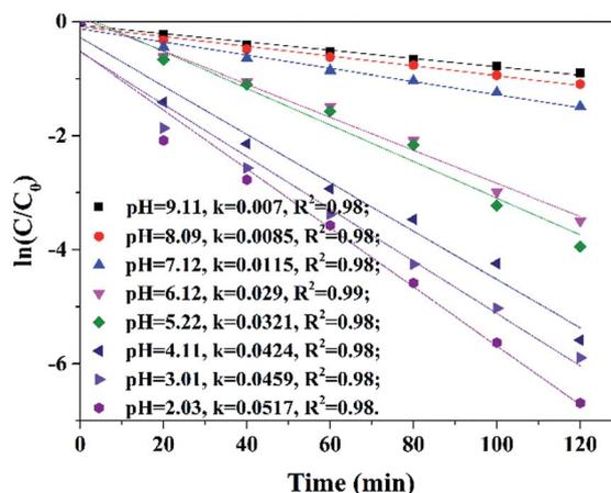
Fig. 9 Pseudo-first-order kinetic curves for AO7 removal under different initial pH values. Reaction conditions: MSDBC dosage =  $1.0 \text{ g L}^{-1}$ ,  $[\text{PS}]_0 = 1.85 \text{ mM}$  and  $[\text{AO7}]_0 = 0.06 \text{ mM}$ .
