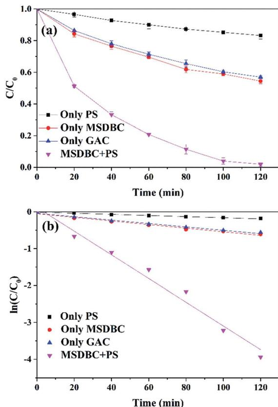
Fig. 5 Degradation and/or adsorption of AO7 by (1) PS (1.85 mM) alone, (2) MSDBC (1 g L<sup>-1</sup>) alone, (3) GAC (1 g L<sup>-1</sup>) alone (4) MSDBC (1 g L<sup>-1</sup>)/PS (1.85 mM). Other reaction conditions: [AO7]<sub>0</sub> = 0.06 mM and pH = 5.22. (a) AO7 removal and (b) pseudo-first-order kinetic curves for AO7 removal.
