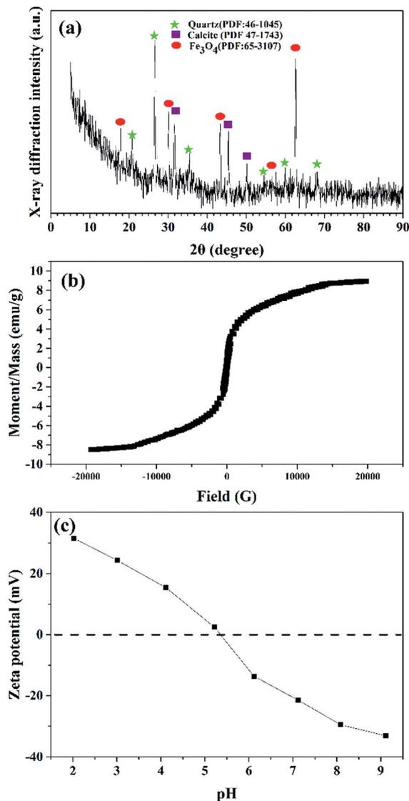
Fig. 1 (a) XRD patterns of MSDBC, (b) magnetization curves measured at room temperature for MSDBC and (c) zeta potentials result of MSDBC.
