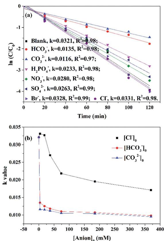
Fig. 10 (a) Effects of common anions on AO7 removal. Reaction conditions:  $[\text{anions}]_0 = 1.85$  mM. (b) Effects of anions concentration on AO7 removal. Reaction conditions:  $[\text{anions}]_0 = 1.85-370$  mM.
