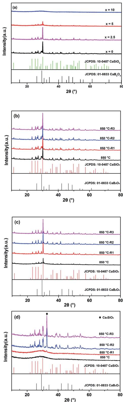
Fig. 7 X-ray diffraction patterns of crystallized glasses at temperature of 850 °C. (a) The patterns glasses isothermally treated one time for  $x = 0, 2.5, 5$  and  $10$ . The patterns of glasses isothermally treated four times (b)  $x = 0$ ; (c)  $x = 5$ ; (d)  $x = 10$ .
