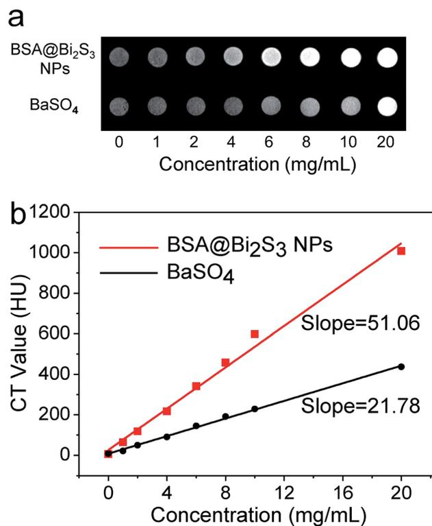
Fig. 2 Comparison of X-ray absorption of BSA@Bi<sub>2</sub>S<sub>3</sub> NPs and BaSO<sub>4</sub> as contrast agents. (a) *In vitro* CT imaging of BSA@Bi<sub>2</sub>S<sub>3</sub> NPs and BaSO<sub>4</sub> at different concentrations (0, 1, 2, 4, 6, 8, 10 and 20 mg mL<sup>-1</sup>) and (b) CT values (HU) of BSA@Bi<sub>2</sub>S<sub>3</sub> NPs and BaSO<sub>4</sub> determined at clinical voltages (80 keV) as a function of mass concentrations of the agents.
