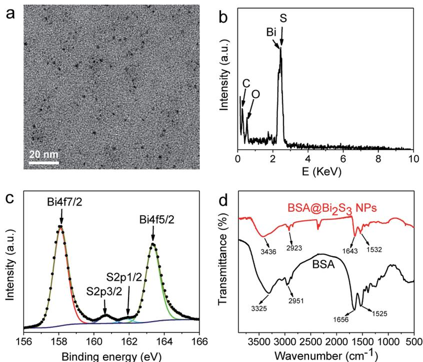
Fig. 1 Characterization of BSA@Bi<sub>2</sub>S<sub>3</sub> NPs. (a) TEM image, (b) EDS spectrum, (c) XPS spectra overlaid with fitting curves for Bi 4f and S 2p, (d) FT-IR spectra.
