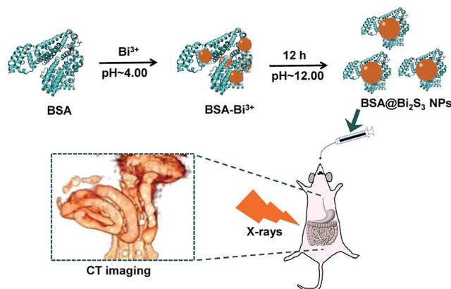
Scheme 1 Schematic illustration of the synthetic routine of BSA@Bi<sub>2</sub>S<sub>3</sub> NPs and their CT imaging of GI tract.
