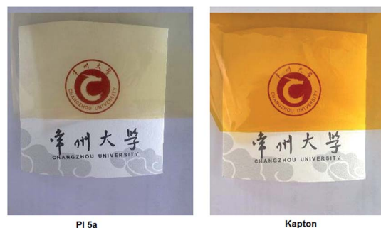
Fig. 8 A comparative image of PI 5a and Kapton.
