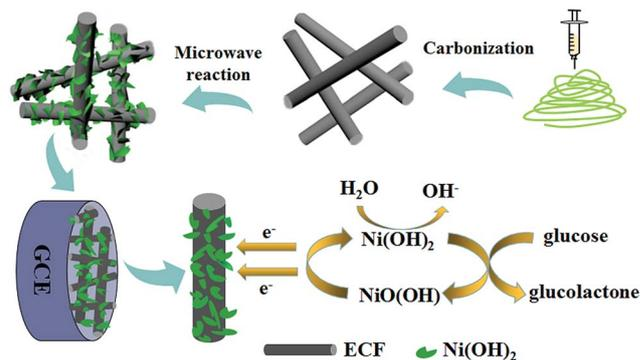
Scheme 1 Construction procedure for Ni(OH)<sub>2</sub>/ECF sensor.
