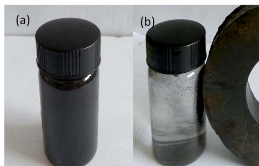
Fig. 12 Digital photographs of RGO/Z/ZF-3 collected by an external magnet (a) before separated; (b) after separated.
