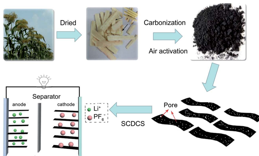
Scheme 1 Schematic illustration of the preparation of SCDCS and the fabrication of SCDCS//SCDCS lithium-ion capacitor.
