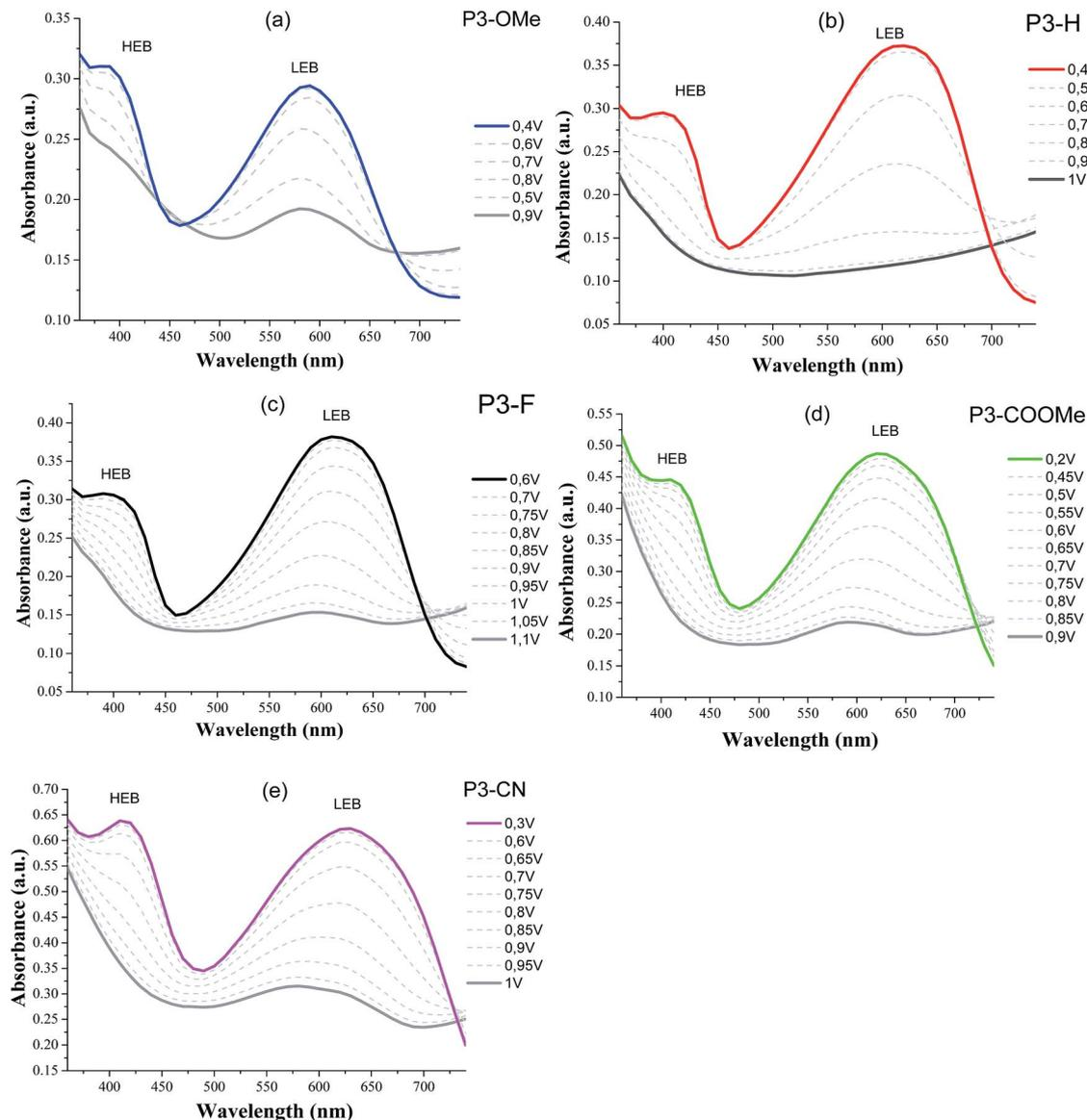
Fig. 5 Spectroelectrochemistry of the polymers on ITO electrode in LiTFSI/ACN (0.1 mol L<sup>-1</sup>) from their coloured state (neutral form) to bleached state (oxidized form). Applied potential are given vs. Ag pseudo-reference.
