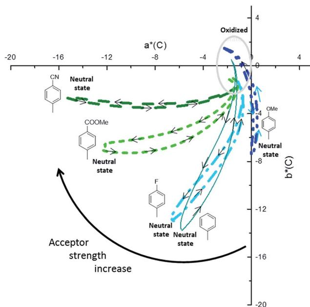
Fig. 6 Colorimetric data obtained from spectroelectrochemical switching study in CIELAB system ( $C/2^\circ$ ) (projected on isosurface color at level  $L^* = 70$ ). P3-OMe (blue, plain line), P3-H (dash), P3-F (dots), P3-COOMe (dash dot), P3-CN (short dot).
