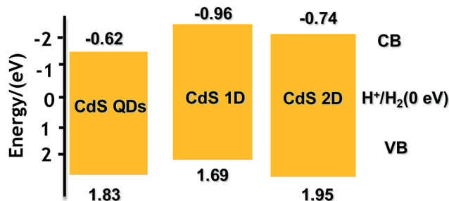
Fig. 6 The band structure alignments of CdS in Pt–ZnS/CdS QDs, Pt–ZnS/CdS 2D, and Pt–ZnS/CdS 1D.
