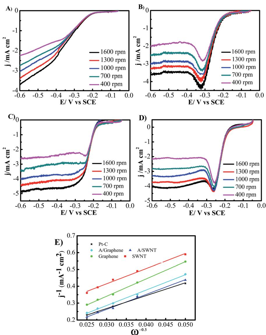
Fig. 7 Linear sweep voltammetry curves of ORR at various rotation rates on (A) SWNT, (B) graphene, (C) A/SWNT, and (D) A/graphene in  $\text{O}_2$ -saturated  $0.1 \text{ M KOH}$  solution with a scan rate of  $10 \text{ mV s}^{-1}$ . (E) The Koutecky–Levich plots at various rotation rates on SWNT, graphene, A/SWNT, and A/graphene and Pt–C electrode at  $-0.45 \text{ V}$  in  $\text{O}_2$ -saturated  $0.1 \text{ M KOH}$  solution. Carbon based materials loading is  $0.25 \text{ mg cm}^{-2}$ .
