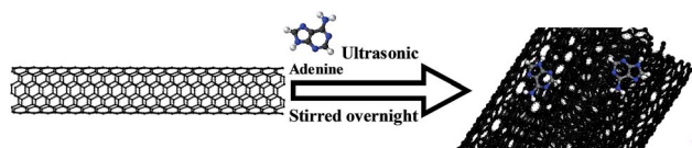
Fig. 1 Schematic of preparation of adenine functionalized carbon nanotubes.
