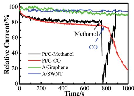
Fig. 8 Chronoamperometry at  $-0.4$  V of Pt/C and adenine functionalized SWNT and graphene in 0.1 M KOH solution with addition of 1 mL methanol and CO. Carbon based materials loading is  $0.25$  mg cm<sup>-2</sup> and Pt–C loading is  $0.05$  mg cm<sup>-2</sup>.
