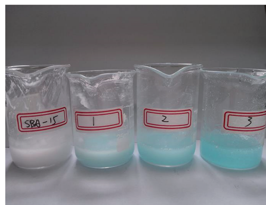
Fig. 10 The photographs of SBA-15 and the precursors corresponding to different catalysts: (1) 0-CCS, (2) 3-CCS, and (3) 5-CCS.
