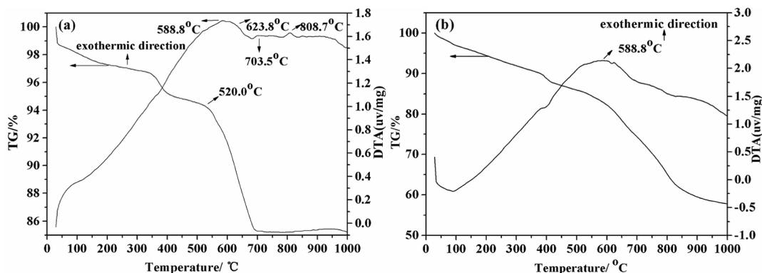
Fig. 1 TG-DTA curve of (a) Kuandian ores and (b) Kuandian ores/ $\text{Na}_2\text{CO}_3$ .
