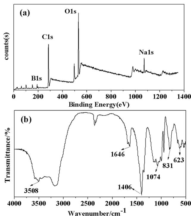
Fig. 4 (a) XPS pattern and (b) FTIR pattern of crystals.
