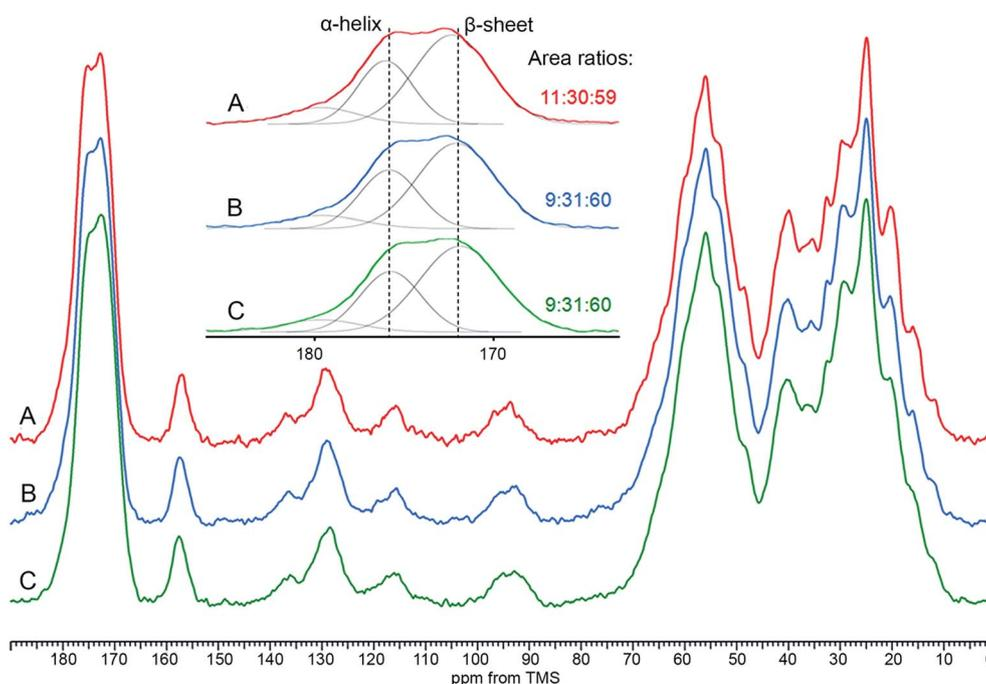
**Fig. 2** The <sup>13</sup>C CP/MAS spectrum of fingernail plates from a single man. (A) Cleaned and cut into snippets, (B) pulverized, (C) pulverized and lyophilized. The inset shows corresponding deconvoluted carbonyl regions with the area ratios of the signals at 179.6, 175.8 and 172.0 ppm.
