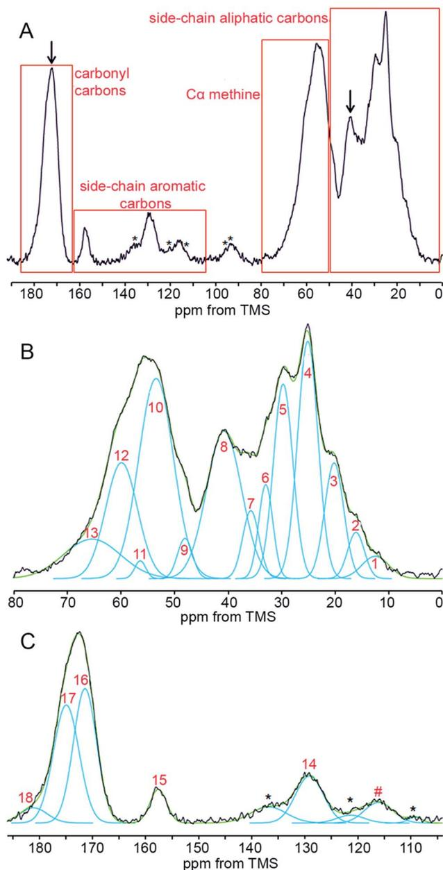
Fig. 1 A typical  $^{13}\text{C}$  CP/MAS NMR spectrum of a human fingernail plate. (A) Full spectrum; (B and C) expanded regions fitted with Gaussian functions. The signal numbers correspond to Table 1. The arrows mark signals that are of particular importance to this work (see text). Asterisks denote spinning sidebands.
