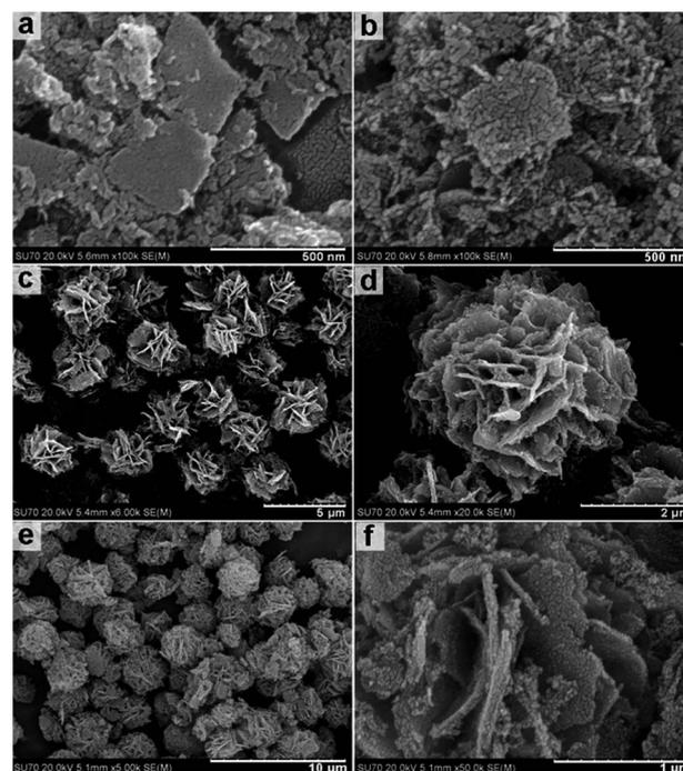
Fig. 2 FESEM images of the sample obtained under solvothermal treatment 160 °C (a) followed by calcination at 400 °C (b); FESEM images of the sample obtained at 180 °C (c & d) followed by the calcination at 400 °C (e & f).
