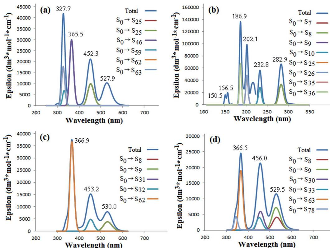
**Fig. 4** Simulated UV-vis absorption spectra and the main corresponding transition composition (a) C<sub>70</sub>, (b) Cor, (c) Cor@C<sub>70</sub>-S and (d) Cor@C<sub>70</sub>-L.
