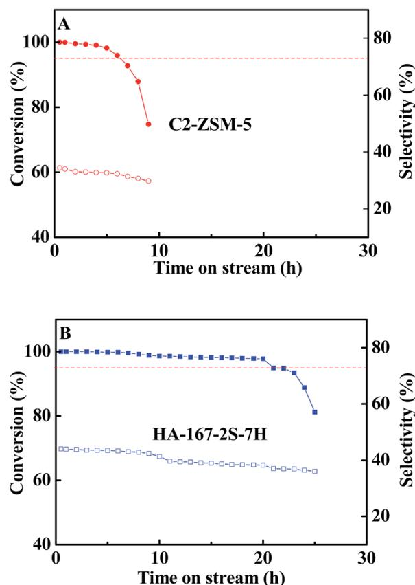
Fig. 11 Conversion of methanol and selectivity of propylene over zeolites C<sub>2</sub>-ZSM-5 (A) and HA-167-2S-7H (B). Reaction conditions: WHSV = 12 h<sup>-1</sup>, T = 470 °C, n(CH<sub>3</sub>OH) : n(H<sub>2</sub>O) = 1 : 1, P = 1 bar.
