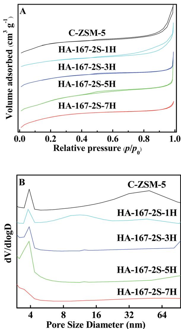
Fig. 5 N<sub>2</sub> adsorption isotherms (A) and PSD curves (B) of the HA-ZSM-5 zeolites with different HTAB/SiO<sub>2</sub> ratios.
