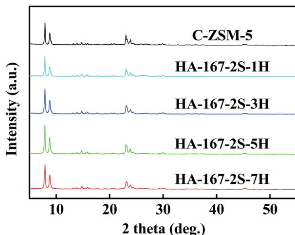
Fig. 6 XRD patterns of the HA-ZSM-5 zeolites synthesized using different HTAB/SiO<sub>2</sub> ratios.
