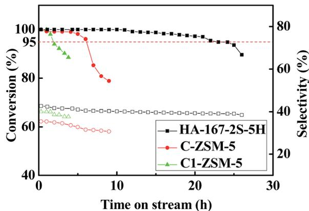
Fig. 10 Methanol conversion and selectivity vs. reaction time:  $T = 470\text{ }^{\circ}\text{C}$ ,  $P = 1\text{ bar}$ ,  $n(\text{methanol}) : n(\text{water}) = 1 : 1$ ,  $\text{WHSV} = 12\text{ h}^{-1}$ .
