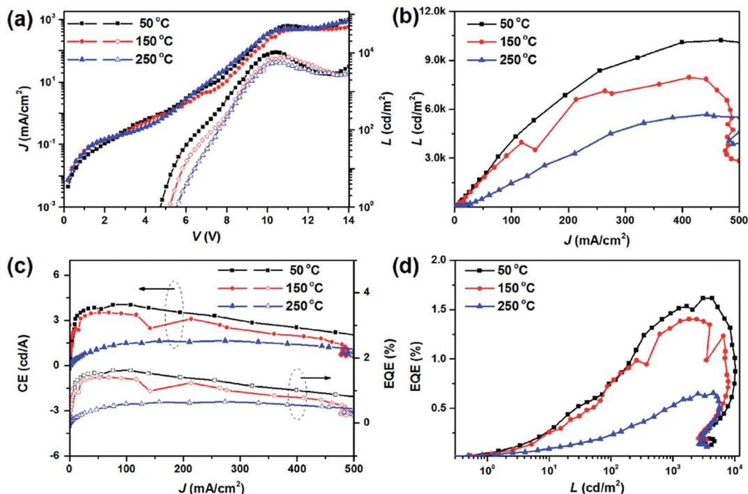
Fig. 6 Characteristics of QD-LEDs with different sMoO<sub>x</sub> HILs annealed at 50 °C, 150 °C and 250 °C, respectively. (a) *J*–*V*–*L* relations; (b) *L* versus *J*; (c) CE versus *J*; (d) EQE versus *L*.
