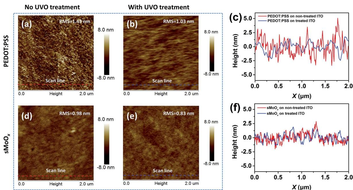
Fig. 2 AFM topological images of PEDOT:PSS films on (a) non-UVO-treated and (b) UVO-treated substrates. (c) The corresponding line scan profiles for the PEDOT:PSS films. AFM images of sMoO<sub>x</sub> films on (d) non-UVO-treated and (e) UVO-treated substrates. (f) Selected line scan profiles for the sMoO<sub>x</sub> films.
