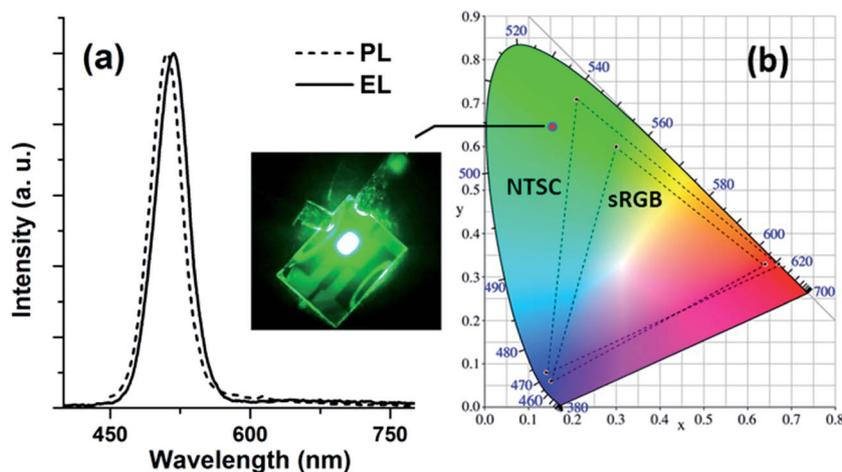
Fig. 9 (a) Comparison of PL emission versus EL spectrum. The inset is an EL image of the sMoO<sub>x</sub>-based QD-LED. (b) Commission Internationale de l'Eclairage (CIE) coordinate for the EL emission.
