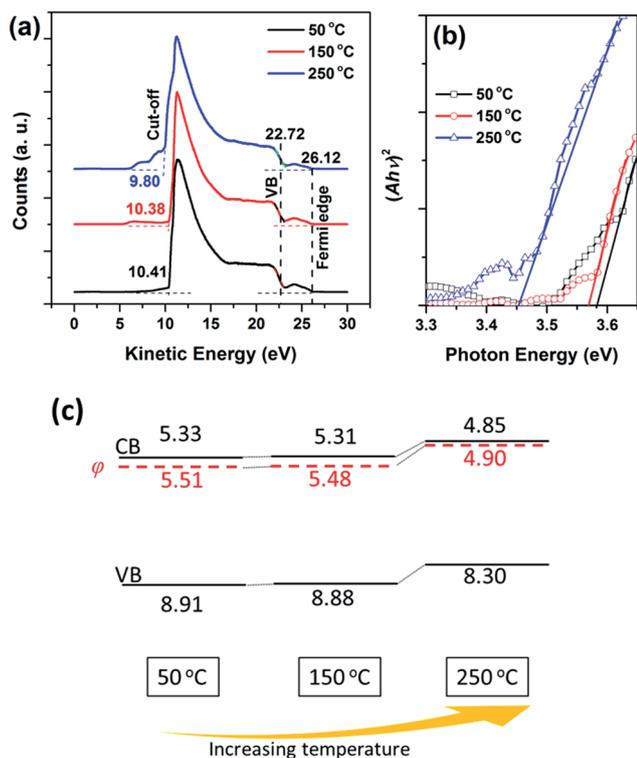
Fig. 7 (a) UPS spectra of  $\text{sMoO}_x$  films after different thermal treatments. (b) Plot of  $(Ah\nu)^2$  versus photon energy for the determination of the optical energy band gap. (c) Band diagram of different  $\text{sMoO}_x$  films.
