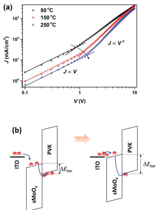
Fig. 8 (a)  $J$ - $V$  characteristics for hole-only devices with a structure of ITO/ $\text{sMoO}_x$ /PVK/QD/ $\text{sMoO}_x$ /Ag. (b) Hole injection behavior of HIL/HTL structure when the  $\text{sMoO}_x$  HIL was annealed at different temperatures.
