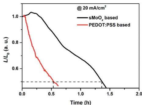
Fig. 5 Operational lifetime characteristics of the resulting sMoO<sub>x</sub>-based and optimized PEDOT:PSS-based QD-LEDs without encapsulation. The devices were operated continuously at a constant current density (20 mA cm<sup>-2</sup>).
