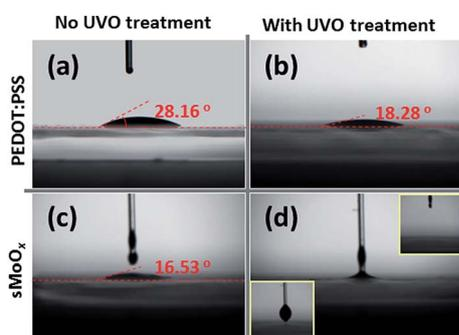
Fig. 1 Contact angles of solutions of PEDOT:PSS and sMoO<sub>x</sub> on ITO-coated glass substrates: (a) PEDOT:PSS on untreated ITO; (b) PEDOT:PSS on UV-ozone-treated ITO; (c) sMoO<sub>x</sub> on untreated ITO; (d) sMoO<sub>x</sub> on UV-ozone-treated ITO. Inset in lower left of the (d) image shows the sMoO<sub>x</sub> droplet before contact and that in the upper right displays a complete wetting for sMoO<sub>x</sub> solution on ITO substrate.
