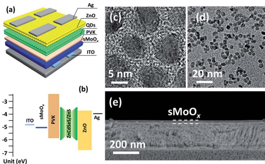
Fig. 3 (a) Device architecture of QD-LED using  $s\text{MoO}_x$  to replace PEDOT:PSS. (b) Flat-band diagram for the multi-layered QD-LED. TEM images of (c) thick-shell ZnCdSeS/ZnS QDs and (d) ZnO NPs. (e) Cross-sectional SEM image of the smooth, uniform  $s\text{MoO}_x$  layer on the ITO substrate.
