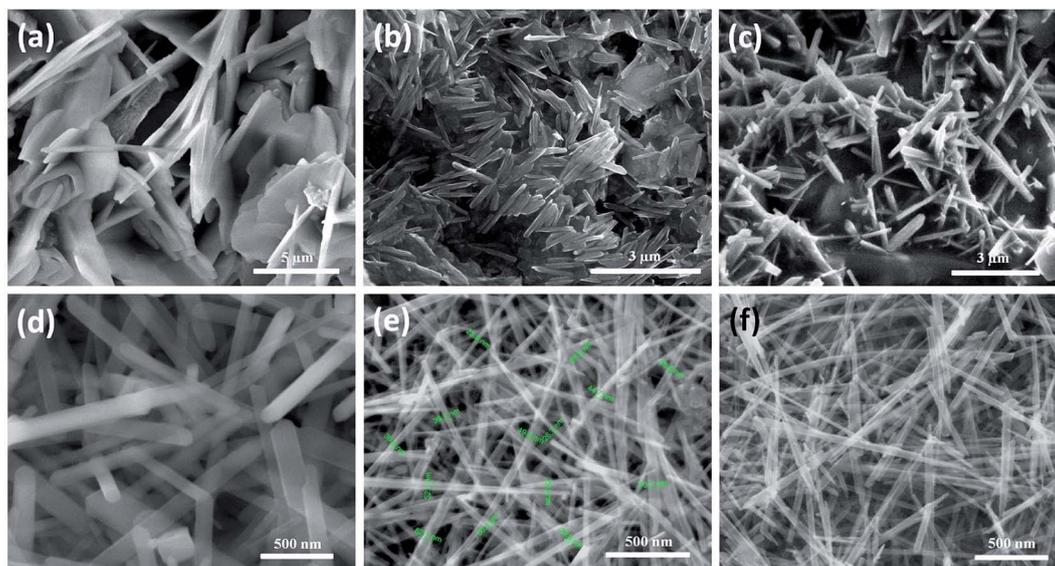
Fig. 3 FESEM images of the final product prepared using  $\text{KMnO}_4$  and  $\text{NaNO}_2$  in the molar ratio of 2 : 3 at a temperature of  $160\text{ }^\circ\text{C}$  for 12 h with  $\text{H}_2\text{SO}_4$  in the molar concentration of (a) 1.3 M, (b) 1.2 M, (c) 0.9 M, (d) 0.6 M, (e) 0.4 M and (f) 0.3 M.
