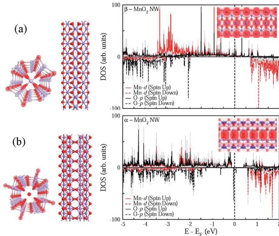
Fig. 5 Calculated quasi-1D nanostructures (top as well as side view) and associated spin-polarized density of states for (a)  $\beta$ -MnO<sub>2</sub> and (b)  $\alpha$ -MnO<sub>2</sub> phases. The electron density difference of each phase for up (red) and down (blue) spins is shown in the respective inset.
