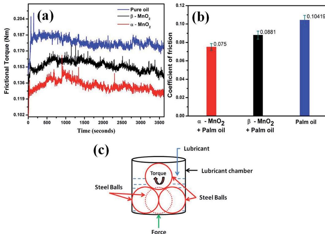
Fig. 6 (a) Frictional torque with respect to time observed using four ball test technique, (b) coefficient of friction of pure palm oil  $\beta$ -MnO<sub>2</sub> added palm oil and  $\alpha$ -MnO<sub>2</sub> added palm oil and (c) schematic outlay of the four-ball test rig.
