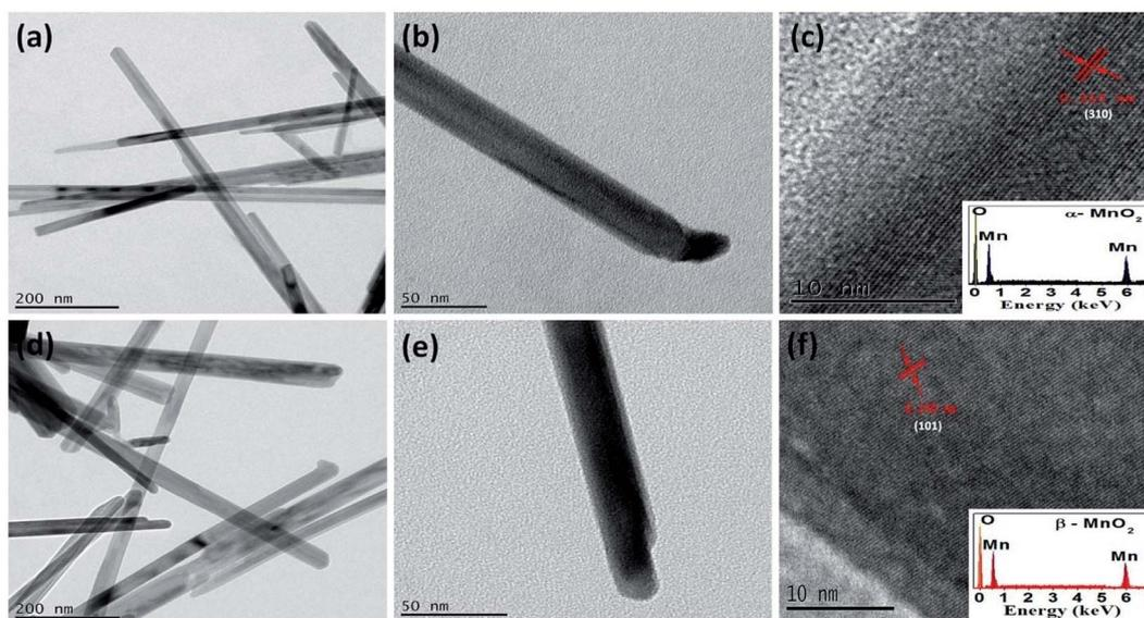
Fig. 2 (a, b) TEM images of  $\alpha$ - $\text{MnO}_2$  at different magnifications, (c) HRTEM image of  $\alpha$ - $\text{MnO}_2$  with growth direction (310),  $d$ -spacing = 0.314 nm and EDX pattern as inset in (c). (d, e) TEM images of  $\beta$ - $\text{MnO}_2$  at different magnifications, (f) HRTEM image of  $\beta$ - $\text{MnO}_2$  with growth direction (101),  $d$ -spacing = 0.24 nm and EDX pattern as inset in (f).
