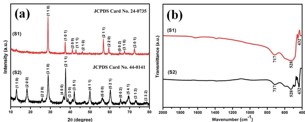
Fig. 1 (a) XRD patterns and (b) FTIR spectroscopy of the samples S1 and S2 prepared using KMnO<sub>4</sub> and NaNO<sub>2</sub> in the molar ratio of 2 : 3 at a temperature of 160 °C for 12 h with H<sub>2</sub>SO<sub>4</sub> in the molar concentration of 0.4 M and 0.3 M, respectively.
