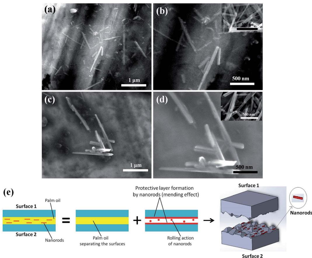
Fig. 8 FESEM images of the deposited nanorods on the scar surfaces of balls tested using (a, b)  $\alpha$ -MnO<sub>2</sub> added palm oil with FESEM image of  $\alpha$ -MnO<sub>2</sub> nanorods as inset in (b), (c, d)  $\beta$ -MnO<sub>2</sub> added palm oil with FESEM image of  $\beta$ -MnO<sub>2</sub> nanorods as inset in (d) and (e) schematic of the mechanisms responsible for enhancement of antiwear property of the base oil by nanorods.
