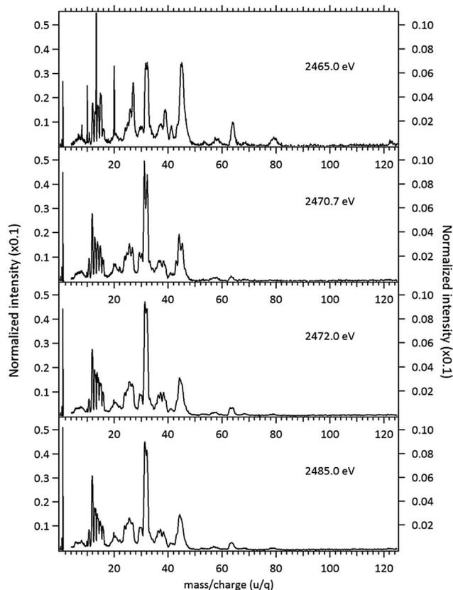
**Fig. 5** Normalized mass spectra of the MPDS molecule obtained below resonances (2465.0 eV), on the resonances (2470.7 eV and 2472.0 eV) and above the S 1s ionization potential (2485.0 eV). The left axis applies only to the intensity of the H<sup>+</sup> ion, while the right axis applies to the intensities of the remaining fragments. The narrow peaks observed at the spectrum obtained below resonances (2465.0 eV) are due to argon contamination ( $m/z = 8; 10; 13.3; 20$ ).
