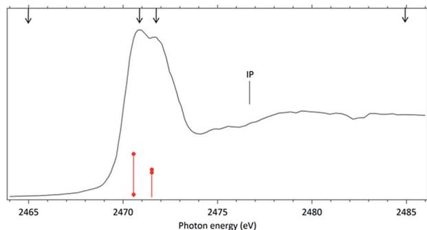
**Fig. 1** Photoabsorption spectrum (NEXAFS) of the DMDS molecule obtained around the S 1s edge. The ionization potential (IP) position was included. The arrows indicate the energy positions in which the TOF spectra were recorded. Calculated values are shown in red, with heights proportional to the oscillator strengths for each transition (red circles).
