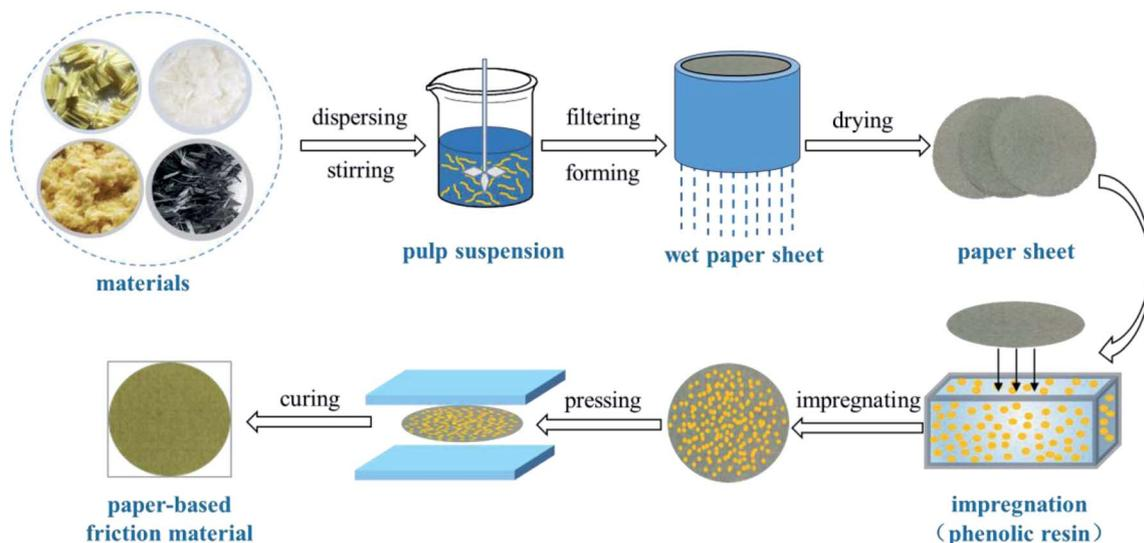
Fig. 1 Schematic illustration for preparing paper-based friction materials.
