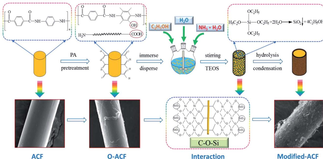
Fig. 2 Schematic illustration for preparing nanosilica-coated ACFs.
