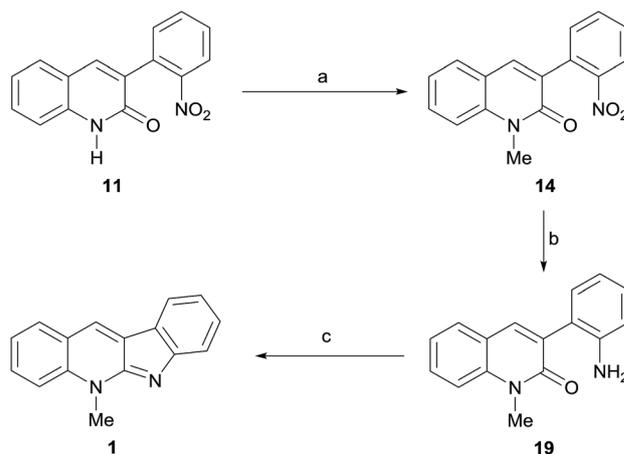
**Scheme 4** Reagents and conditions: (a) DMC, DMF, DBU, 90 °C, overnight (95%); (b) Fe, NH<sub>4</sub>Cl, EtOH–H<sub>2</sub>O (9 : 1, v/v), reflux, 3 h (96%); (c) 1. POCl<sub>3</sub>, MeCN, 90 °C, overnight; 2. DIPEA, 120 °C, overnight (63%).
