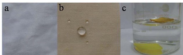
Fig. 4 (a) Unmodified cellulose fabric absorbs the water. (b) The modified PT-CF shows the rolling water droplet on the surface. (c) The modified PT-CS sponge shows the buoyancy property on the water surface whereas the unmodified cellulose sponge sinks within seconds.
