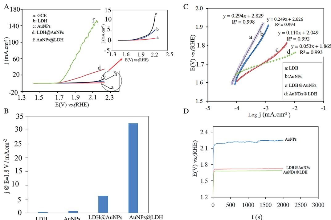
Fig. 3 OER polarization curves of the electrodes at a scan rate of  $5 \text{ mV s}^{-1}$  (A), current densities of the electrodes at a fixed potential of 1.80 V vs. RHE (B), OER Tafel plots (C), and chronopotentiometric curves at  $0.032 \text{ mA cm}^{-2}$  (D), in 1.0 M KOH solution.
