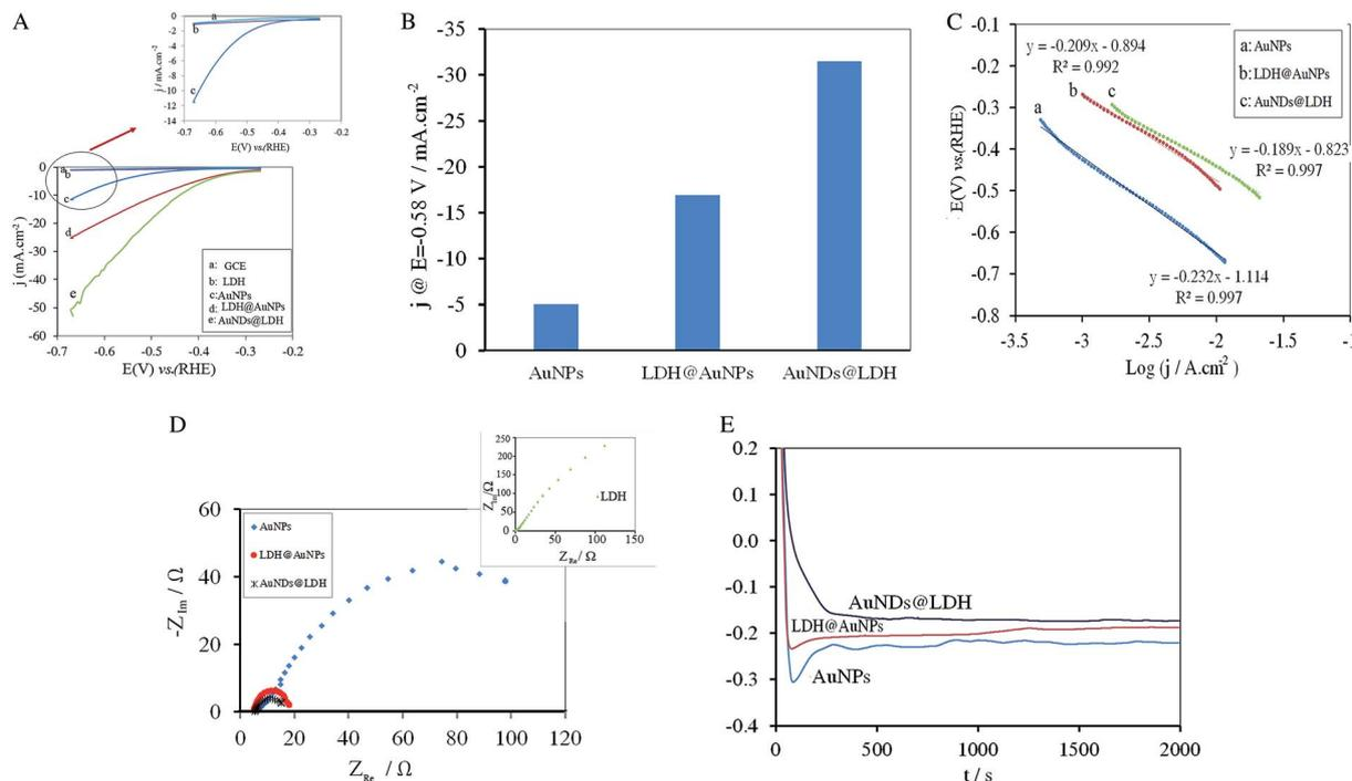
Fig. 4 HER polarization curves of the electrodes at a scan rate of 5 mV s<sup>-1</sup> (A), current densities of the electrodes at a fixed potential of -0.58 V vs. RHE (B), HER Tafel plots (C), Nyquist plots at -1.60 V (D), and chronopotentiometric curves under a constant current density of -0.016 mA cm<sup>-2</sup> (E), in 1.0 M KOH solution.
