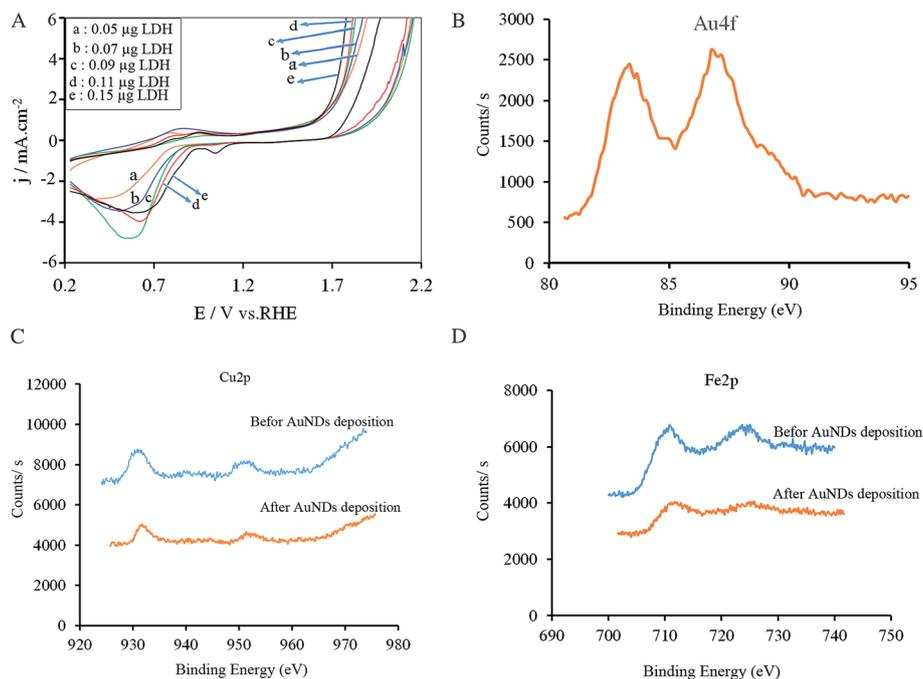
Fig. 5 Cyclic voltammograms of the AuNDs@LDH/GCE with different amounts of LDH in 1.0 M KOH at scan rate of 50 mV s<sup>-1</sup> (A); and XPS spectrums for Au (B), Cu (C), and Fe (D).
