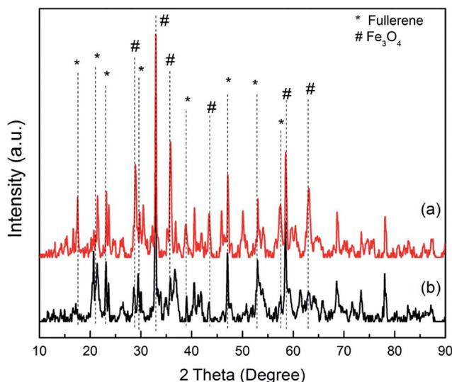
Fig. 1 XRD spectrum of (a) fullerene/Fe<sub>3</sub>O<sub>4</sub> (FMNPs) and (b) β-CD-fullerene/Fe<sub>3</sub>O<sub>4</sub> (CDFMNPs) nanocomposite.
