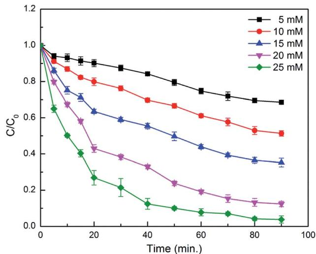
Fig. 8 Effect of  $\text{H}_2\text{O}_2$  on degradation of alizarin by CDFMNPs, reaction conditions: catalyst =  $2.0 \text{ g L}^{-1}$ , pH = 3, [alizarin] =  $10 \text{ mM}$  at room temperature. The experiments were performed in triplicate and error bars show the standard deviation for the analyses.
