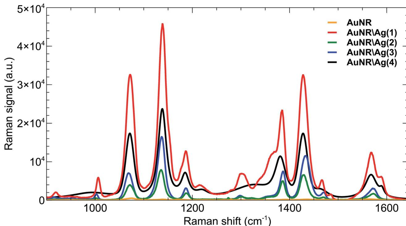
Fig. 5 SERS signals from Raman agents with bare gold nanorods (AuNRs) and gold nanorods with 1, 2, 3 and 4 nm silver thicknesses (AuNR\Ag(1-4)).
