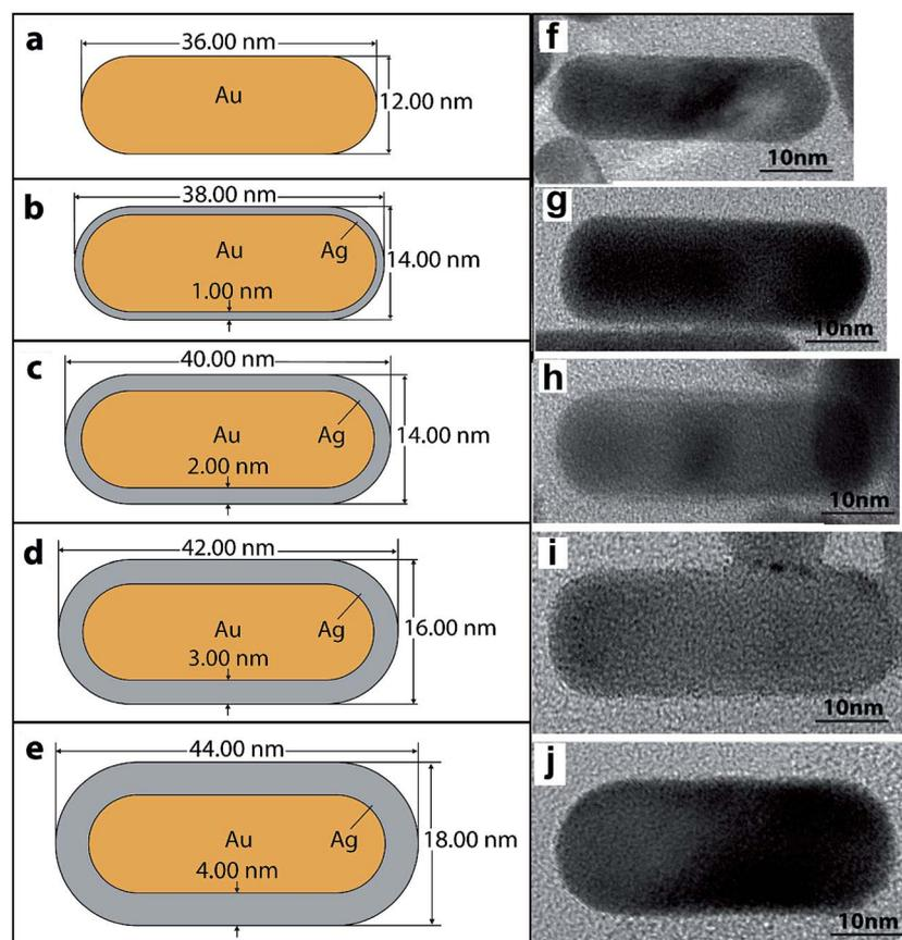
Fig. 2 The dimensions of the AuNRs and AuNR\Ags with 0, 1, 2, 3, and 4 nm silver shells and 12  $\times$  36 nm gold cores that were used in the numerical model, (a–e) respectively. (f–j) HRTEM images: (f) a gold nanorod only, and (g–j) gold nanorods covered with (1, 2, 3, and 4 nm) silver shells, respectively.
