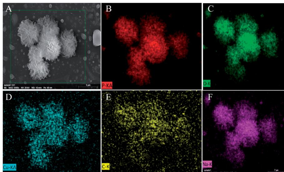
Fig. 2 (A) SEM image of SC-Cu<sub>3</sub>(PO<sub>4</sub>)<sub>2</sub>·3H<sub>2</sub>O nanoflowers. SEM element mapping analyses of nanoflowers: (B) P, (C) O, (D) Cu, (E) C, (F) Na.
