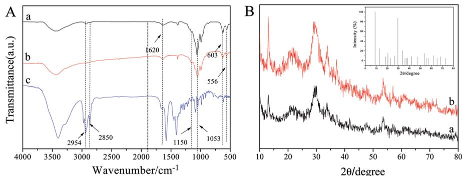
Fig. 3 (A) FT-IR spectra of (a) SC- $\text{Cu}_3(\text{PO}_4)_2 \cdot 3\text{H}_2\text{O}$  nanoflowers; (b)  $\text{Cu}_3(\text{PO}_4)_2$ ; (c) SC; (B) XRD patterns of (a)  $\text{Cu}_3(\text{PO}_4)_2$  and (b) SC- $\text{Cu}_3(\text{PO}_4)_2 \cdot 3\text{H}_2\text{O}$  nanoflowers, inset is the standard card of  $\text{Cu}_3(\text{PO}_4)_2 \cdot 3\text{H}_2\text{O}$  (JPCSD00-022-0548).
