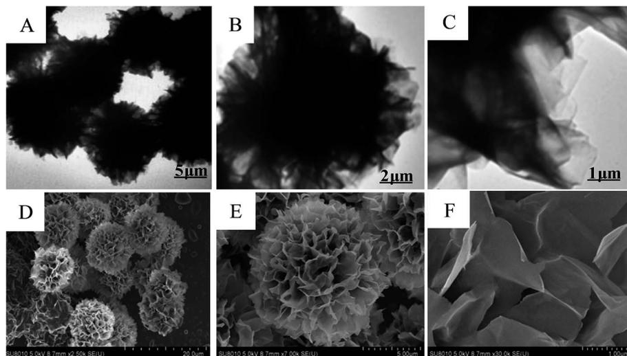
Fig. 1 The detailed characterizations of SC-Cu<sub>3</sub>(PO<sub>4</sub>)<sub>2</sub>·3H<sub>2</sub>O nanoflowers (0.1 mg mL<sup>-1</sup> SC). TEM image of (A) hybrid nanoflowers, (B) a local partial enlarged image of (A), and (C) nanopetals (a local partial enlarged image of (B)). SEM images of (D) hybrid nanoflowers, (E) single nanoflower (a local partial enlarged image of (D)) and (F) nanopetals (a local partial enlarged image of (E)).
