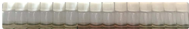
Fig. 7 Photographs of F-6 in methanol/H 2 O (8 : 2) solution and followed by the addition of metal ions (from left to right: blank sample, Na + , K + , Ba 2+ , Mg 2+ , Ca 2+ , Al 3+ , Fe 3+ , Cu 2+ , Pb 2+ , Zn 2+ , Cd 2+ , Ni 2+ , Co 2+ , Mn 2+ ).
