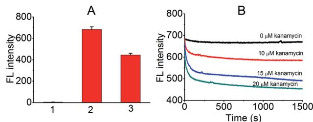
Fig. 2 ThT FL analysis for the kanamycin A induced FL displacement biosensor. (A) Depicts the ThT FL in different states. Column 1 = 1  $\mu\text{M}$  ThT, 2 = 1  $\mu\text{M}$  ThT + 1  $\mu\text{M}$  KanaApt, and 3 = 2 + 20  $\mu\text{M}$  kanamycin A. (B) Shows the real-time fluorescence when different concentrations of kanamycin A (0 to 20  $\mu\text{M}$ ) were added to the 1  $\mu\text{M}$  KanaApt–ThT complex.
