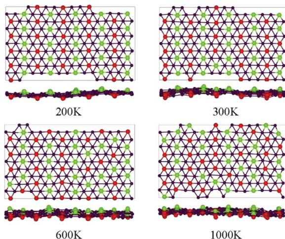
Fig. 2 Snapshots for the equilibrium structures of  $\text{BeB}_2$  monolayer ( $\delta$  phase) at the temperatures of 200 K, 300 K, 600 K, and 1000 K, at the end of 2 ps *ab initio* molecular dynamics simulations. The label of the atoms is the same as in Fig. 1.
