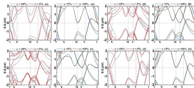
**Fig. 6** The band structures of four structures ( $\alpha$ ,  $\beta$ ,  $\gamma$ ,  $\delta$ ) of  $\text{BeB}_2$  monolayer under biaxial strains  $\varepsilon = -10\%$ ,  $-5\%$ ,  $5\%$  and  $10\%$ .
