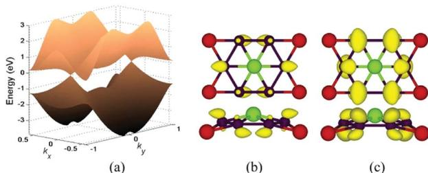
**Fig. 5** (a) The 3D band structure of  $\delta$  phase under 3.2% biaxial tensile strain, which has Dirac point located at the Fermi level. Band decomposed charge density of  $\text{BeB}_2$  monolayer of (a) at Dirac point: the projection of the charge density of the highest valence band (b) and the lowest conduction band (c). The isosurface value was set at  $0.21 a_0^{-3}$  and  $0.13 a_0^{-3}$  ( $a_0$ : Bohr radius) respectively.
