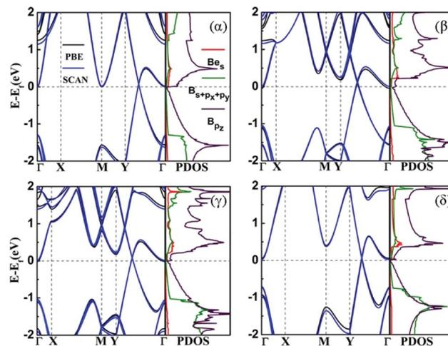
Fig. 3 The band structures and projected density of states (PDOS) of four structures ( $\alpha$ ,  $\beta$ ,  $\gamma$ ,  $\delta$ ). The black lines in band structures and the PDOS were calculated by PBE functional, while the blue lines in band structures were calculated by SCAN functional.
