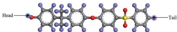
Fig. 1 The chemical structure for a polysulfone repeated single chain; purple: hydrogen, grey: carbon, yellow: sulphur, red: oxygen atom.
