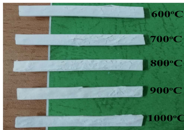
Fig. 6 Self-supporting of ceramifying silicone rubber composites.
