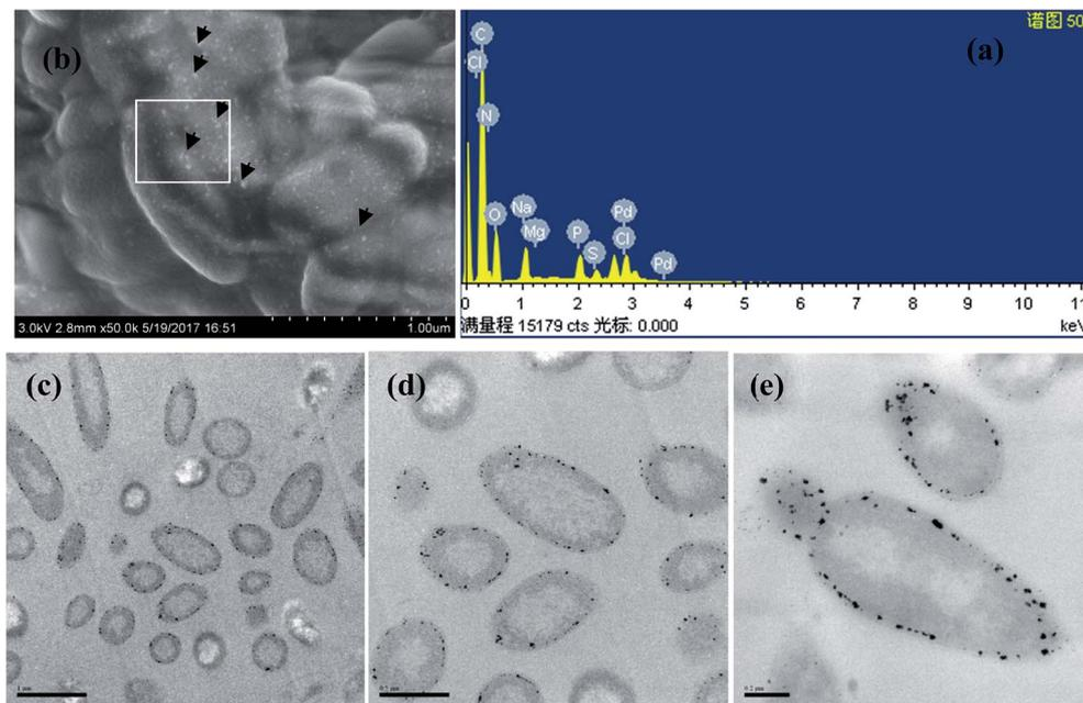
Fig. 2 SEM image of Pd attached CNZ-1 cells (24 h) (a); EDX image of the marked area in (a) and (b); TEM image of Pd attached CNZ-1 cells with different scale accuracy: 1  $\mu\text{m}$  (c), 0.5  $\mu\text{m}$  (d) and 0.2  $\mu\text{m}$  (e).
