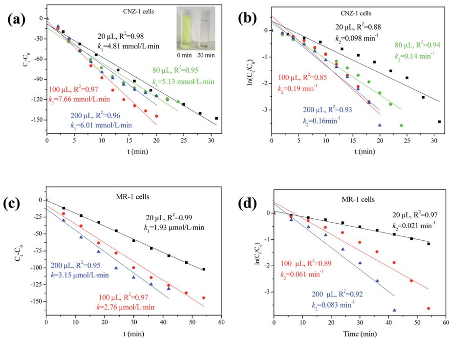
Fig. 7 4-NP reduction mediated by  $\text{bio}_{\text{CNZ-1}}\text{-Pd}^0$  (a, b) and  $\text{bio}_{\text{MR-1}}\text{-Pd}^0$  (c, d) with different concentrations in the presence of  $\text{NaBH}_4$ ; plots of  $C_t - C_0$  vs. time (a, c) and  $\ln(C_t/C_0)$  vs. time (b, d) for the reduction of 4-NP by  $\text{NaBH}_4$ .
