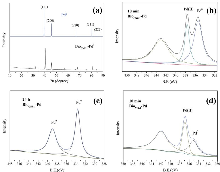
Fig. 3 The XRD spectra of  $\text{bio}_{\text{CNZ-1}}\text{-Pd}^0$  (a); the XPS spectra (Pd 3d) of  $\text{bio}_{\text{CNZ-1}}\text{-Pd}^0$  at 10 min (b) and 24 h (c); the XPS spectra (Pd 3d) of  $\text{bio}_{\text{MR-1}}\text{-Pd}^0$  at 10 min (d).
