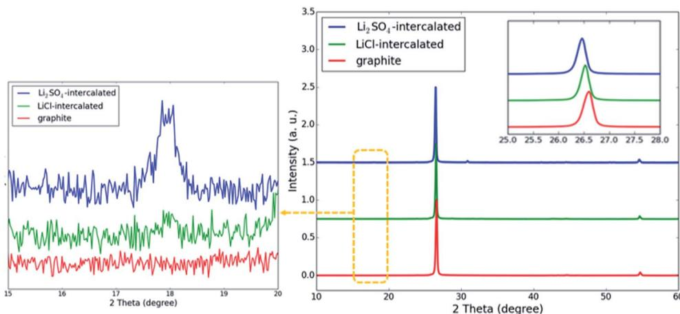
Fig. 9 XRD patterns of inorganic salt-intercalated graphite obtained by  $\text{Li}_2\text{SO}_4$  and LiCl intercalation. The inset image shows the shift of the (002) peak and the left image shows the diffraction peaks near  $18^\circ$ .
