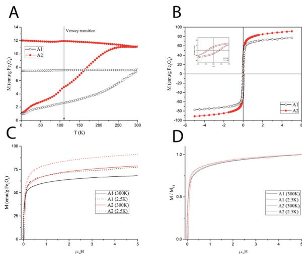
**Fig. 2** (A) ZFC and FC magnetization curves acquired by applying a 5 mT probing field; (B) hysteresis cycles at  $T = 2.5\text{ K}$ ; (C)  $M(H)$  curves measured at 2.5 and 300 K; (D)  $M(H)$  curves measured at 2.5, and 300 K normalized to the 5 T value. All the data were collected on dry powders of samples A1 and A2 and are reported per gram of magnetic material,  $\text{Fe}_3\text{O}_4$ , evaluated from ICP-MS data.
