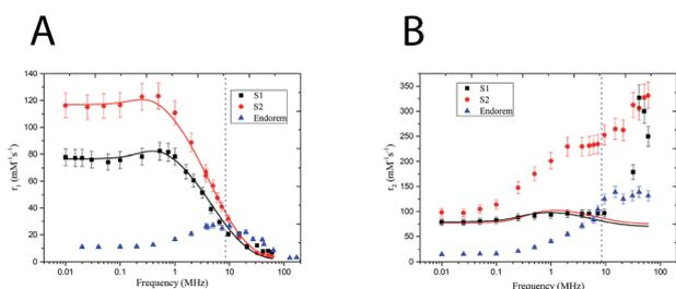
Fig. 3 Nuclear magnetic relaxation dispersion (NMRD)  $r_1$  (A) and  $r_2$  (B) profiles for samples S1, S2 compared to the commercial compound, Endorem. The dashed lines represent the frequencies used in MRI images. The solid lines are the best-fitting to the experimental data (see text for details).
