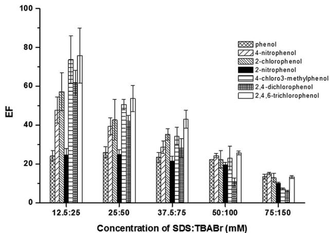
Fig. 1 Effect of SDS. Conditions: sample solution; 10 mL,  $\text{AlCl}_3$ ; 5% (w/v), vortex agitation time; 30 s, centrifugation time (3500 rpm); 10 min, the mole ratio of SDS : TBABr; 1 : 2 and  $50 \mu\text{g L}^{-1}$  of each phenol.
