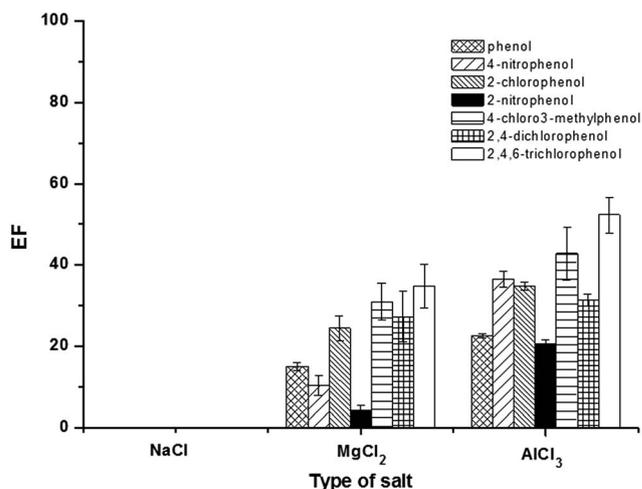
Fig. 3 Effect of type of salt. Conditions: sample solution; 10 mL, SDS;  $25 \text{ mmol L}^{-1}$ , TBABr;  $75 \text{ mmol L}^{-1}$ , salt; 5% (w/v), vortex agitation time; 30 s, centrifugation time (3500 rpm); 10 min and  $50 \mu\text{g L}^{-1}$  of each phenol.
