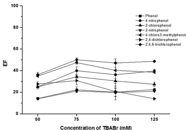
Fig. 2 Effect of TBABr. Conditions: sample solution; 10 mL, SDS;  $25 \text{ mmol L}^{-1}$ ,  $\text{AlCl}_3$ ; 5% (w/v), vortex agitation time; 30 s, centrifugation time (3500 rpm); 10 min and  $50 \mu\text{g L}^{-1}$  of each phenol.
