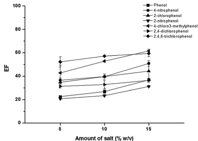
Fig. 4 Effect of amount of salt. Conditions: sample solution; 10 mL, SDS; 25 mmol L<sup>-1</sup>, TBABr; 75 mmol L<sup>-1</sup>, vortex agitation time; 30 s, centrifugation time (3500 rpm); 10 min and 50 μg L<sup>-1</sup> of each phenol.
