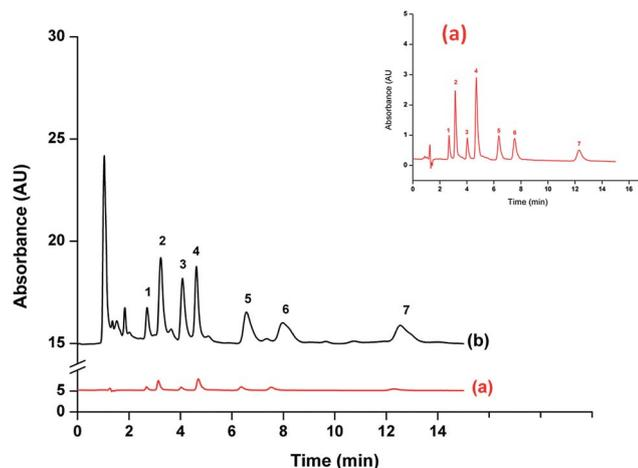
Fig. 5 Typical chromatograms of (a) without preconcentration (500 μg L<sup>-1</sup> of Ph, 4NP, 2CP and 2NP and 1000 μg L<sup>-1</sup> of 4C3MP, 2,4DCP and 2,4,6TCP) and (b) after the proposed extraction method (25 μg L<sup>-1</sup> of 4NP and 2NP and 50 μg L<sup>-1</sup> of Ph, 2CP, 4C3MP, 2,4DCP and 2,4,6TCP). Peak; 1 = Ph, 2 = 4NP, 3 = 2CP, 4 = 2NP, 5 = 4C3MP, 6 = 2,4DCP and 7 = 2,4,6TCP.
