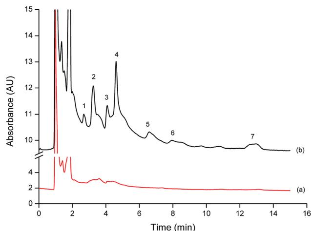
Fig. 6 Typical chromatograms of agricultural water sample extracted by the proposed method; (a) blank sample and (b) spiked sample with  $15 \mu\text{g L}^{-1}$  of the studied phenols. Peak: 1 = Ph, 2 = 4NP, 3 = 2CP, 4 = 2NP, 5 = 4C3MP, 6 = 2,4DCP and 7 = 2,4,6TCP.
